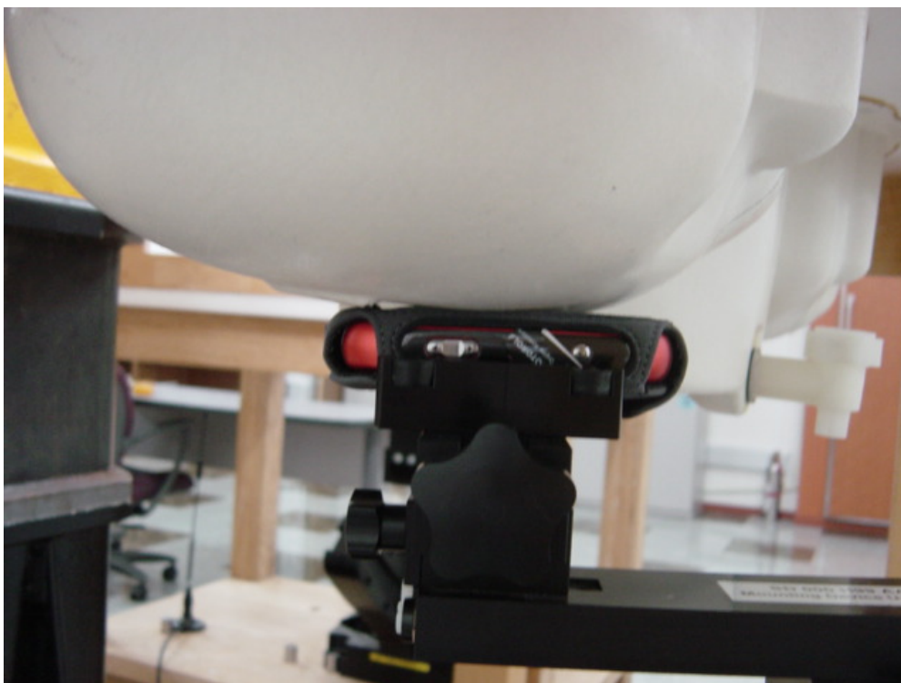
Figure 5. Phone with Arm Band Case SYN1697A Against the Head Phantom (Cheek Touch)
