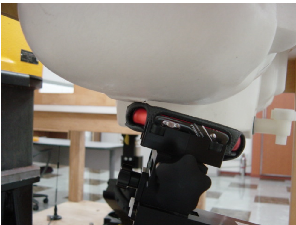
Figure 6. Phone with Arm Band Case SYN1697A Against the Head Phantom (15°Tilt)
