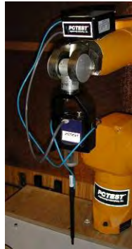
Figure 10 SPEAG Robotic System
