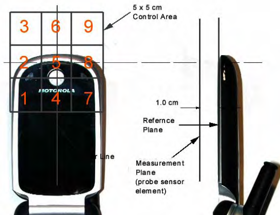
Figure 13 E/H-Field Emissions Test Setup Diagram
