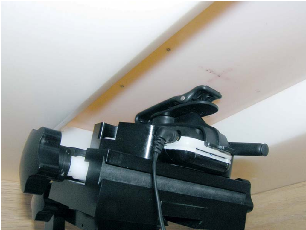
Figure 19. Phone in Holster Against the Flat Phantom with Antenna Retracted
