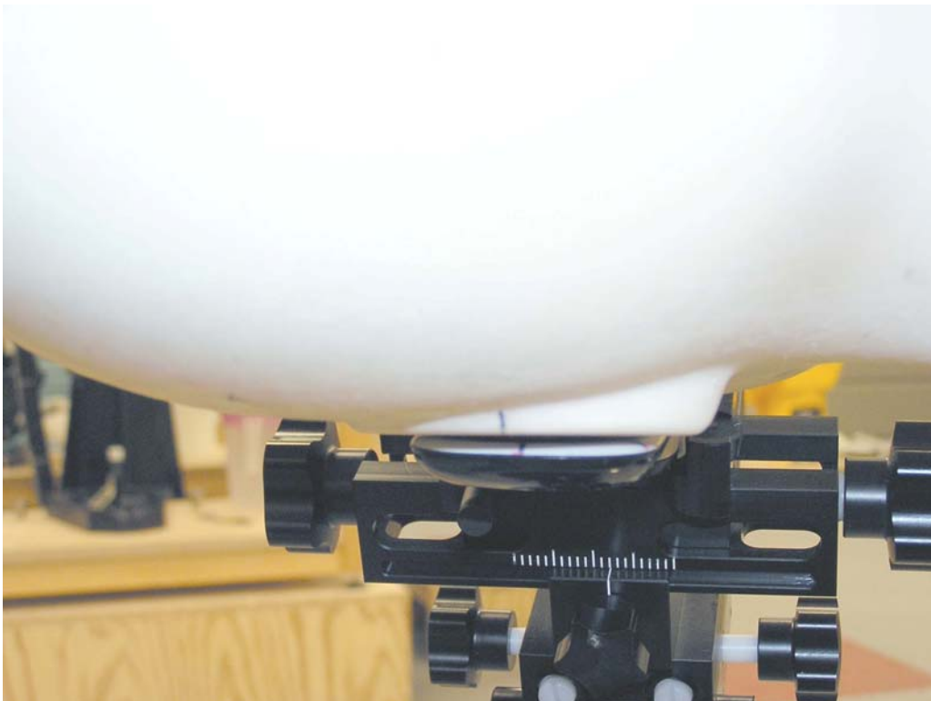
Figure 12. Phone Against the Head with Antenna Retracted (Back View – Cheek Touch)
