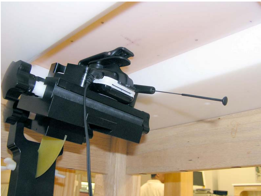
Figure 20. Phone in Holster Against the Flat Phantom with Antenna Extended
