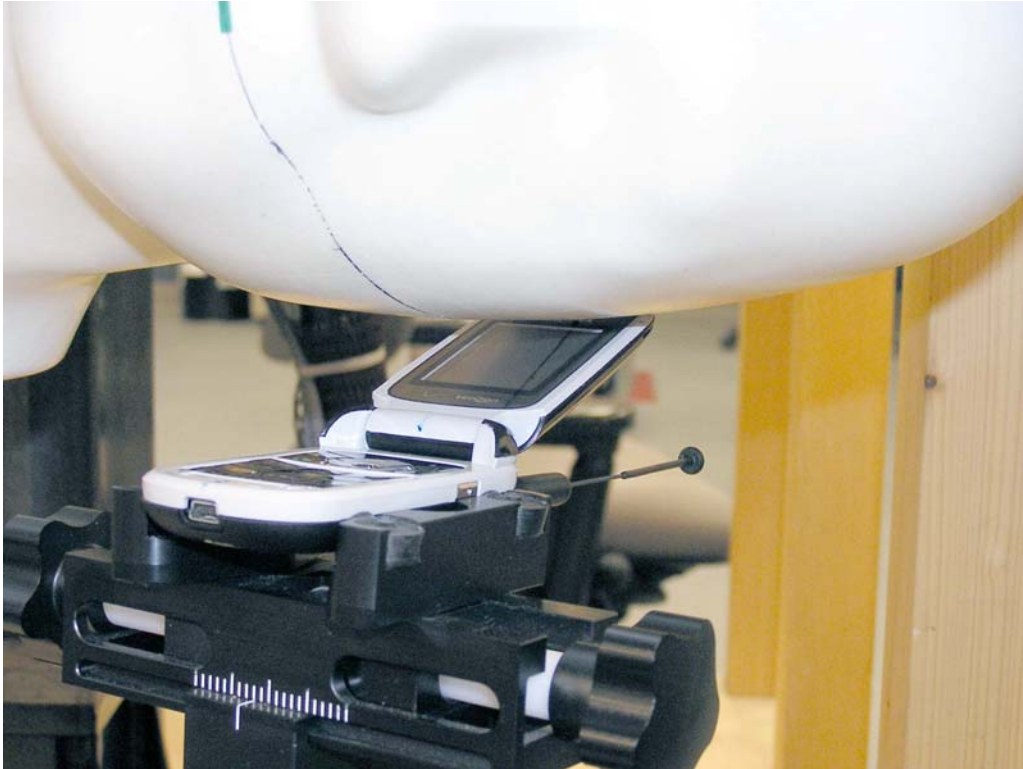
Figure 17. Phone Against the Head with Antenna Extended (Front View – 15°Tilt)
