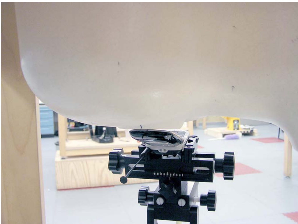
Figure 18. Phone Against the Head with Antenna Extended (Back View – 15°Tilt)
