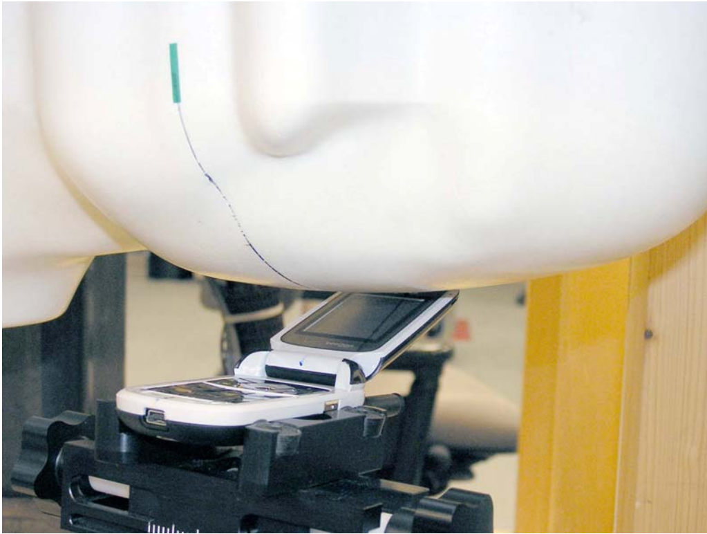
Figure 15. Phone Against the Head with Antenna Retracted (Front View – 15°Tilt)
