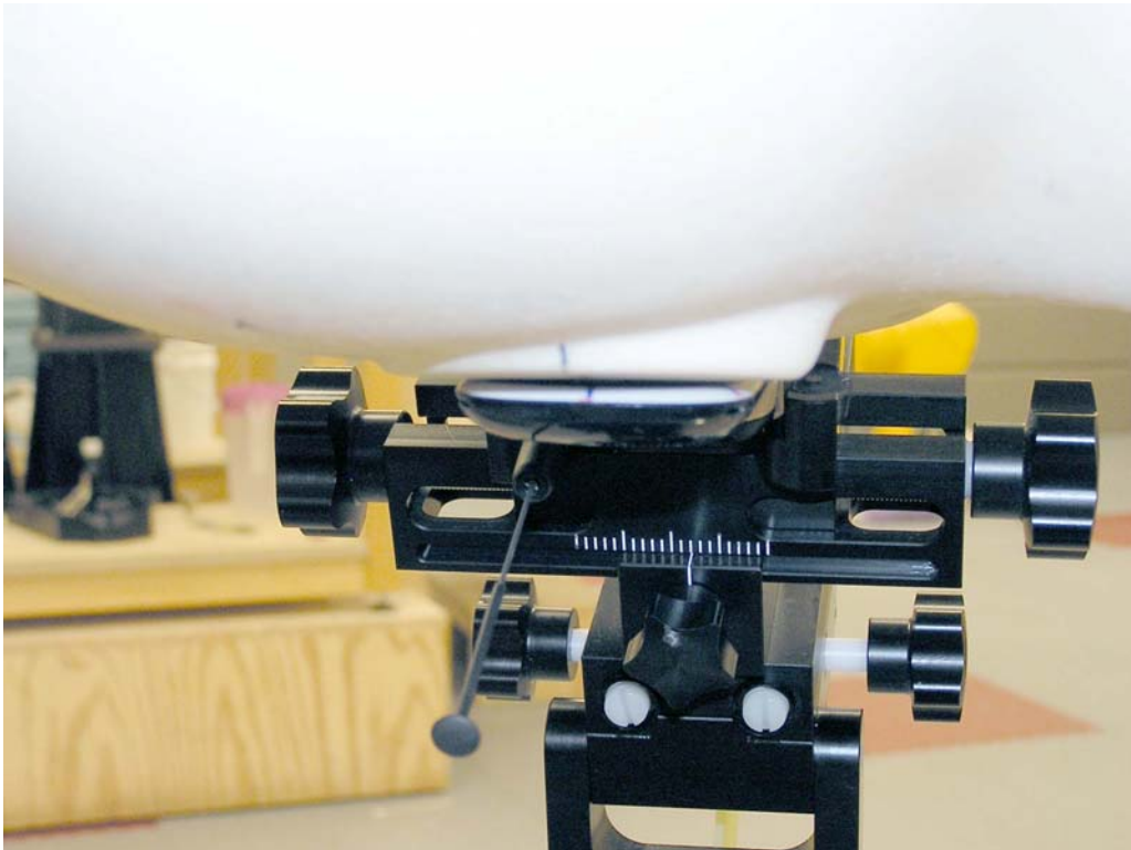
Figure 14. Phone Against the Head with Antenna Extended (Back View – Cheek Touch)
