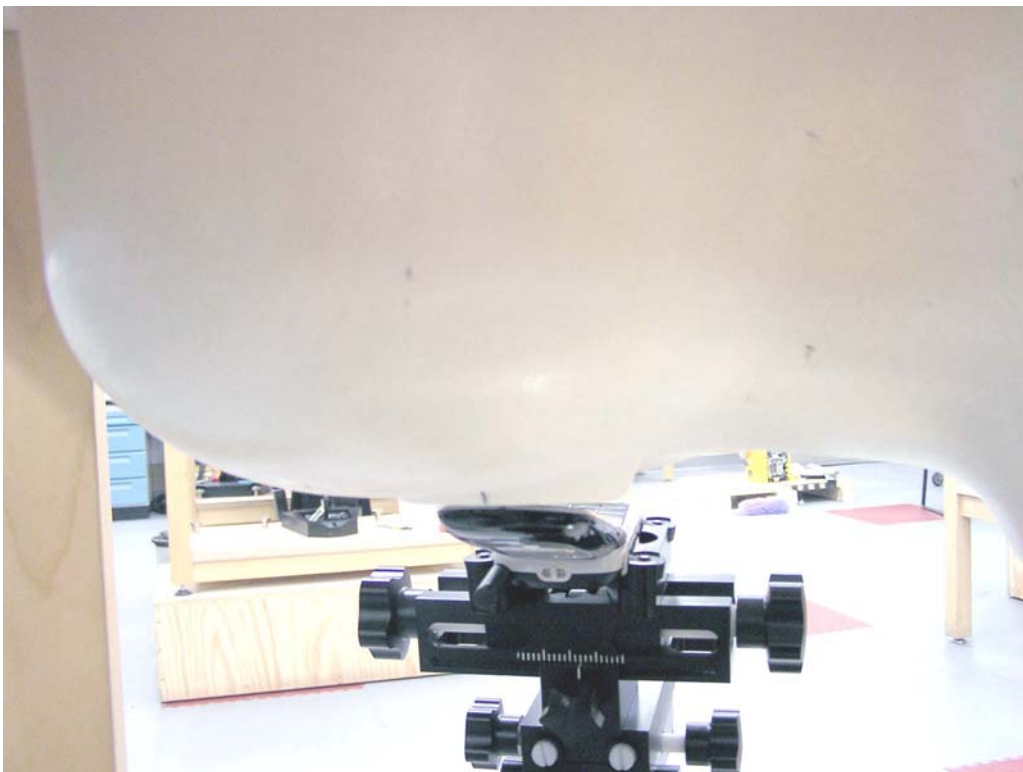
Figure 16. Phone Against the Head with Antenna Retracted (Back View – 15°Tilt)
