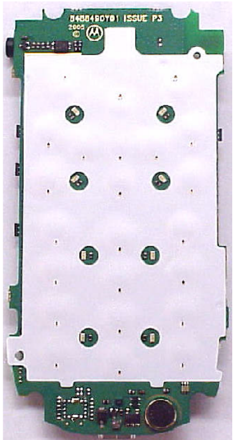
Main Board (keypad installed)
