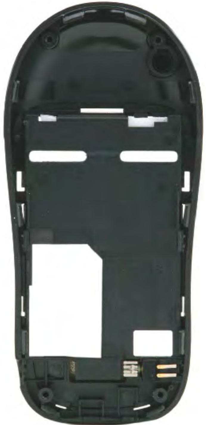
Rear Housing Internal View
