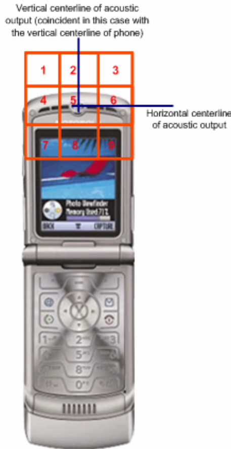
Figure 2: Orientation of Wireless Device and Measurement Plane
