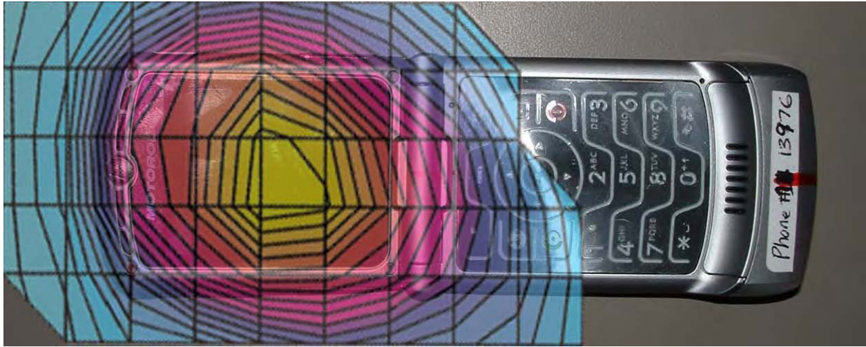
Figure 3. Typical 850MHz GSM Head Adjacent Contour Overlaid on Phone (15 ° Tilt)
