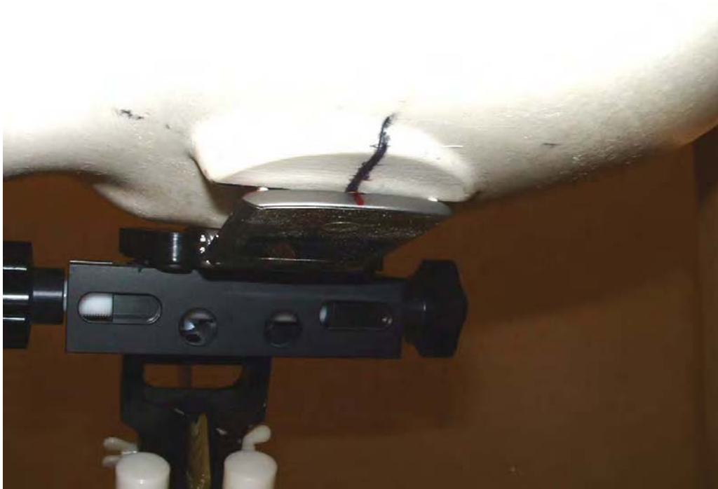
Figure 11. Rear View; Cheek/Touch Position
