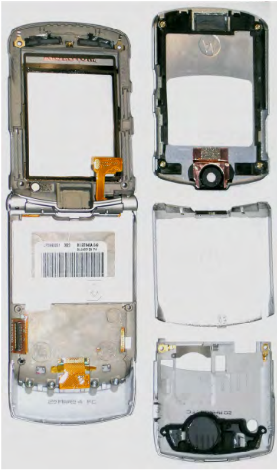
Housing Internal View
