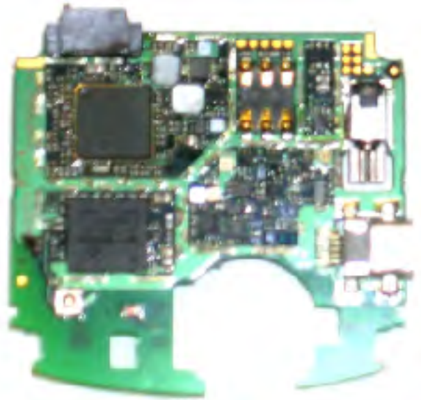
Front View (Shields Removed)
