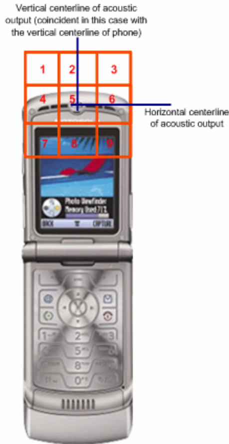
Figure 2: Orientation of Wireless Device and Measurement Plane
