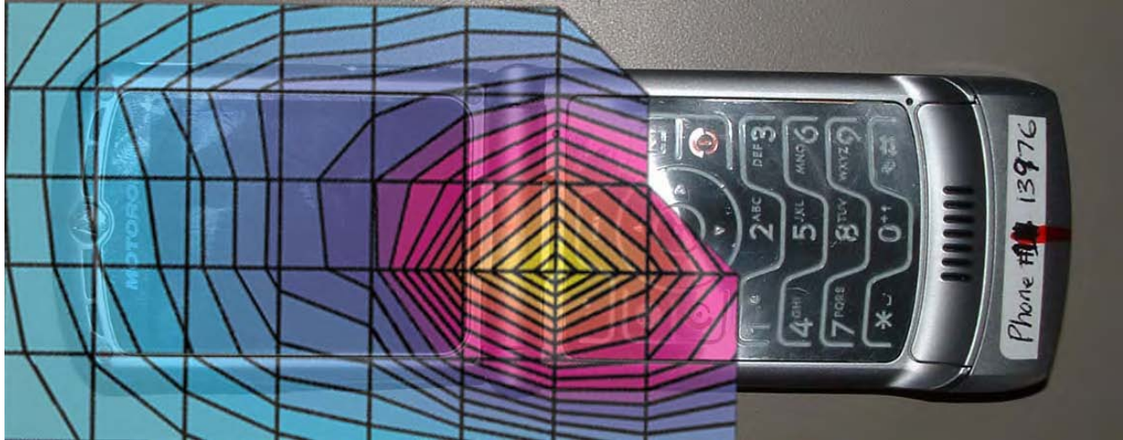
Figure 1. Typical 850MHz GSM Head Adjacent Contour Overlaid on Phone (Cheek Touch)
