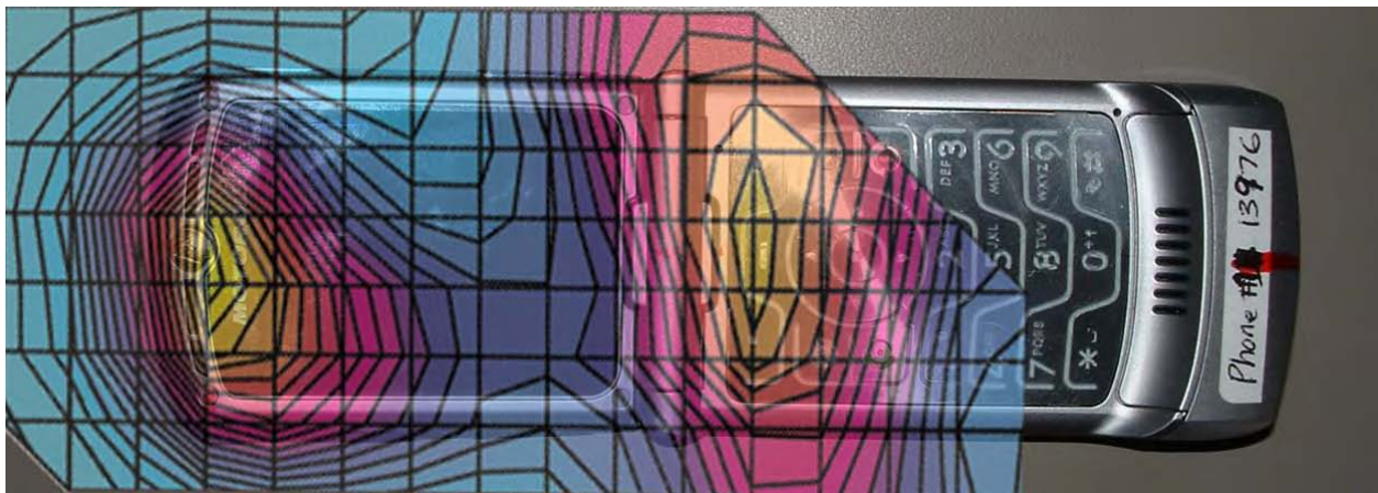
Figure 4. Typical 1900MHz GSM Head Adjacent Contour Overlaid on Phone (15 ° Tilt)
