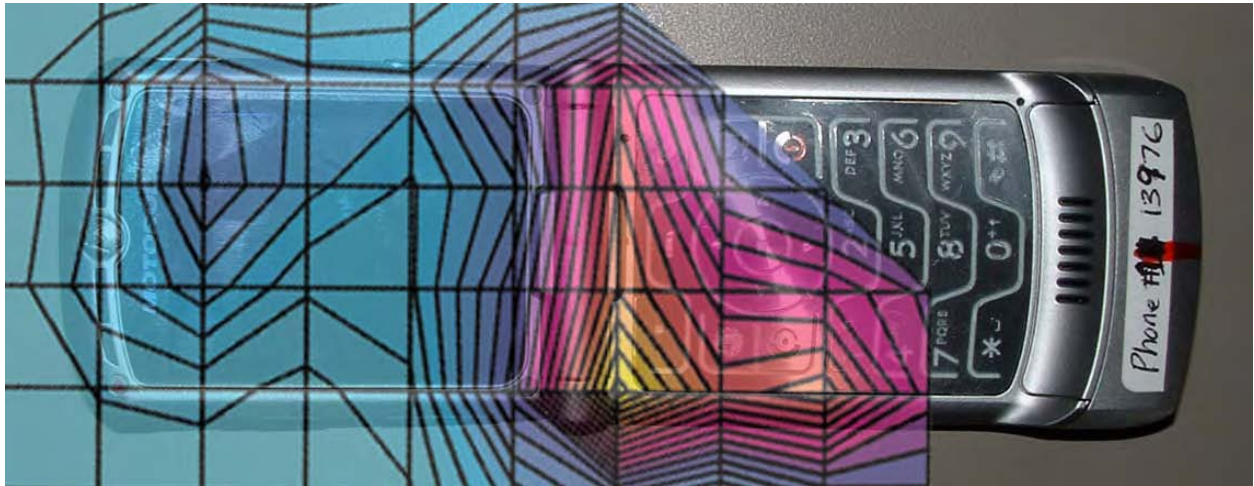
Figure 5. Typical Bluetooth Head Adjacent Contour Overlaid on Phone (Cheek Touch)
