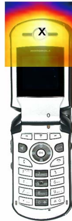
Figure 27 Sample E-field Scan Overlay
