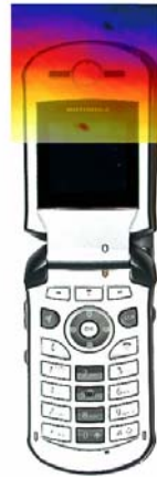
Figure 28 Sample H-field Scan Overlay
