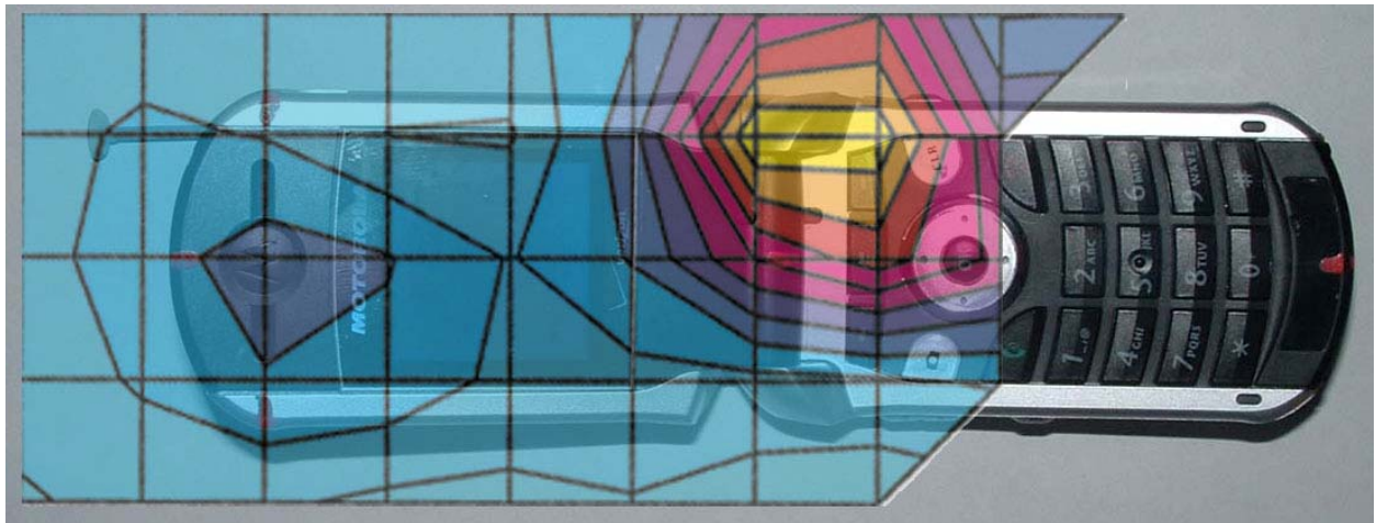
Figure 4. Typical 1900MHz Head Adjacent Contour Overlaid on Phone with Antenna Extended (Cheek Touch)
