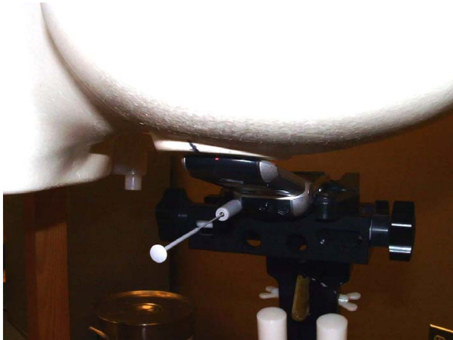
Figure 28. Phone Against the Head with Antenna Extended (Back View – 15°Tilt)
