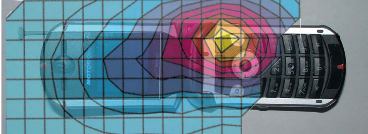
Figure 1. Typical 800MHz Head Adjacent Contour Overlaid on Phone with Antenna Extended (Cheek Touch)
