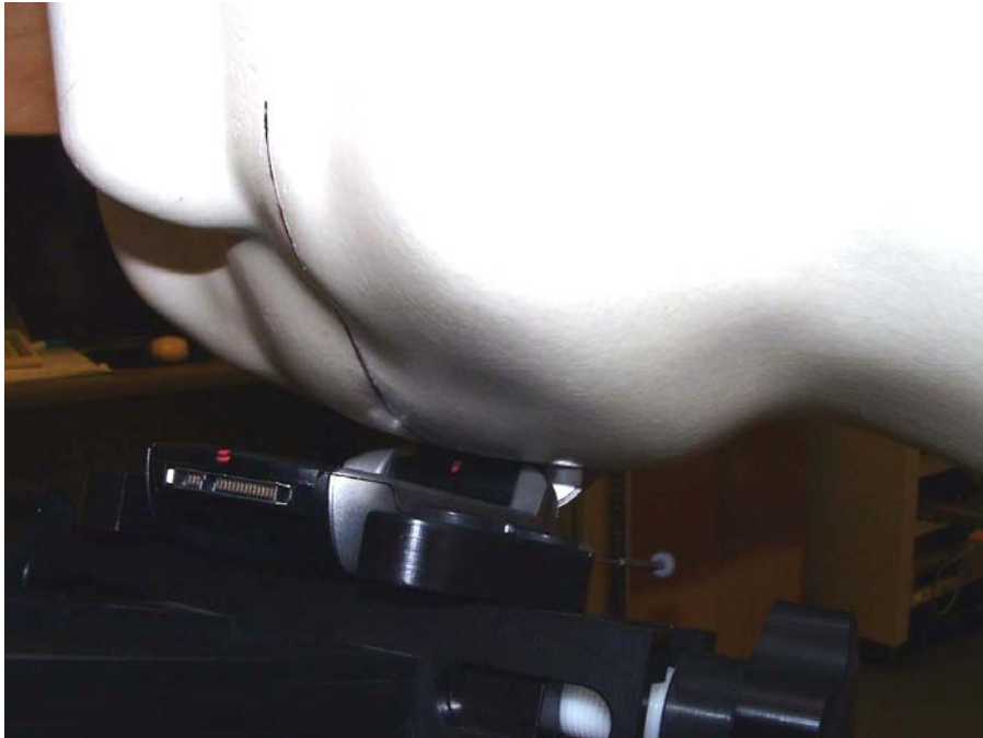
Figure 23. Phone Against the Head with Antenna Extended (Front View – Cheek Touch)
