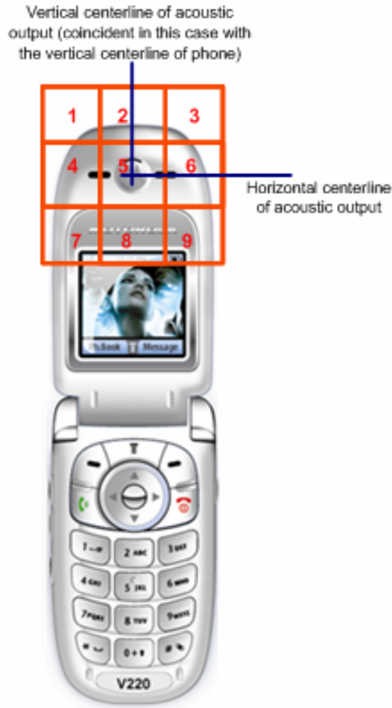
Figure 2: Orientation of Wireless Device and Measurement Plane
