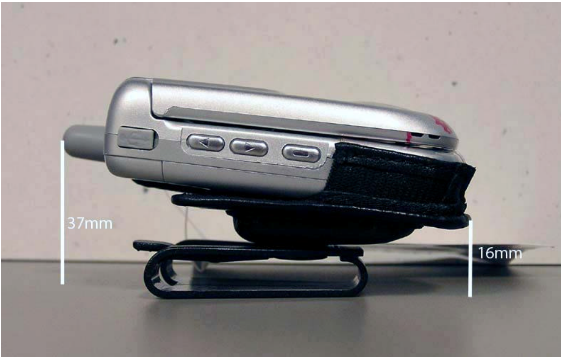
Figure 3. Side of Phone with SYN8631A Clip
