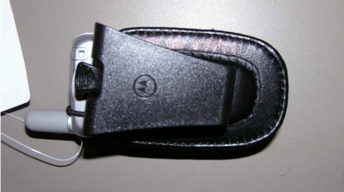
Figure 2. Back of Phone with SYN8631A Clip
