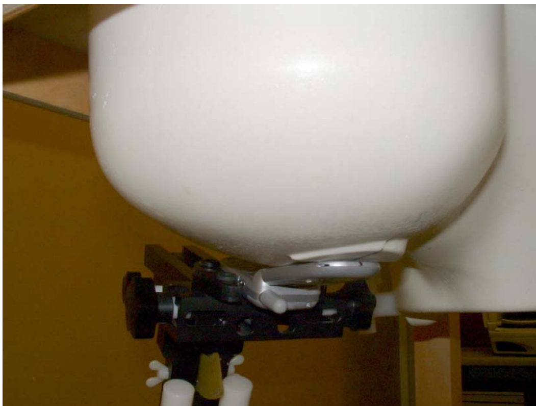
Figure 11. Phone Against the Head Phantom (Back View – Cheek Touch)
