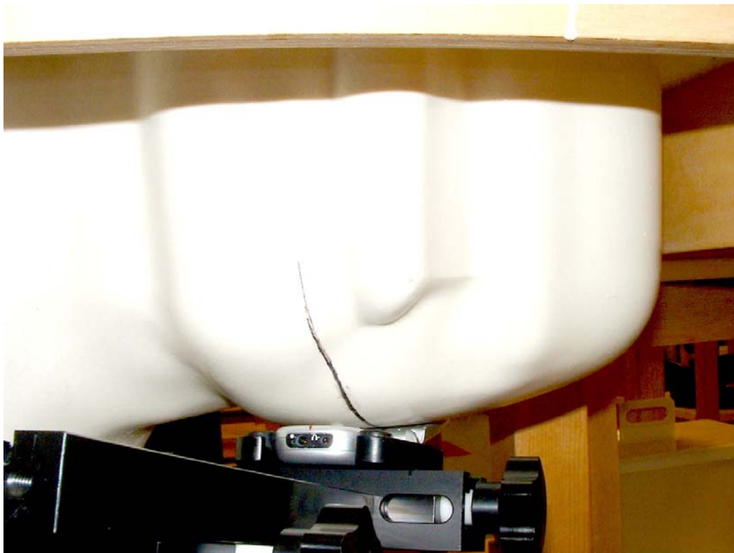
Figure 10. Phone Against the Head Phantom (Front View - Cheek Touch)
