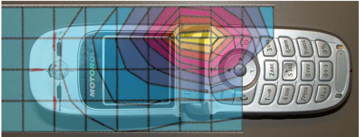
Figure 1. Typical 850MHz Head Adjacent Contour Overlaid on Phone (Cheek Touch)
