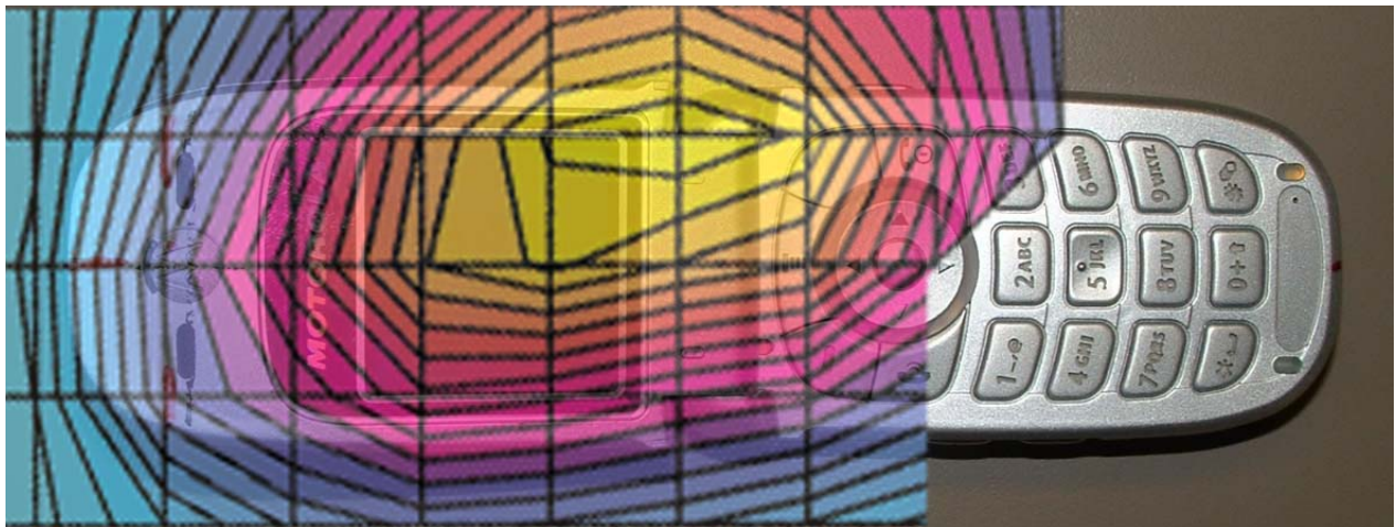
Figure 2. Typical 850MHz Head Adjacent Contour Overlaid on Phone (15° Tilt)
