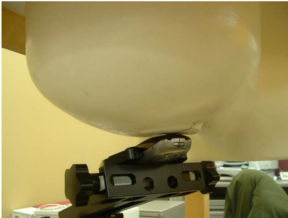
Phone Placed Against Phantom Head in 15 Degree Tilt Position (rear view)
