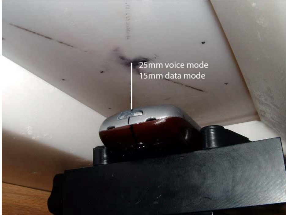
Phone with No Available Body-worn Cases Positioned Below Phantom
