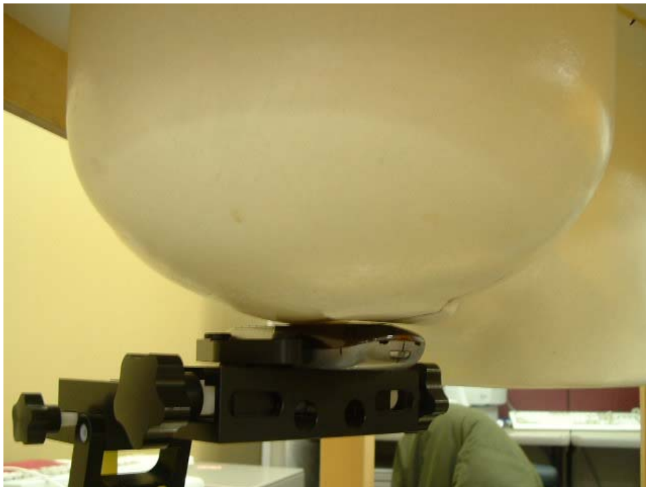
Phone Placed Against Phantom Head in Check Touch Position (rear view)
