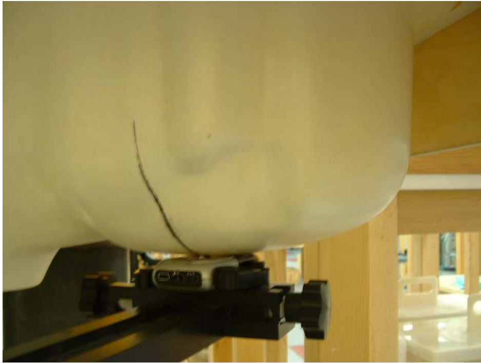
Phone Placed Against Phantom Head in Check Touch Position (front view)
