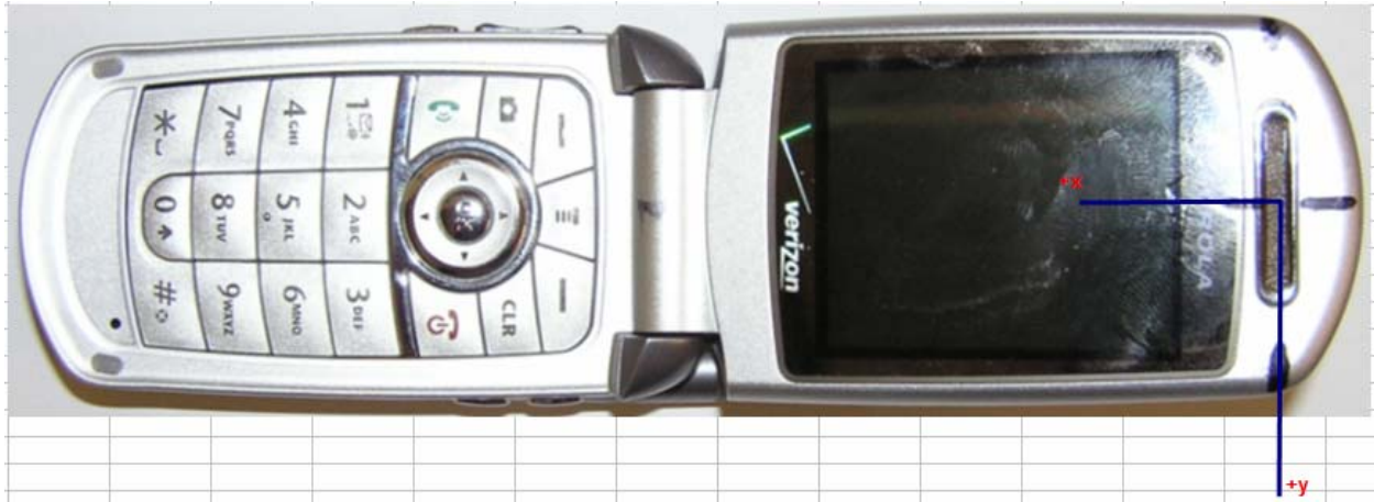
Figure A3-4. Phone Open – Coordinate Axis for T-coil Measurements
