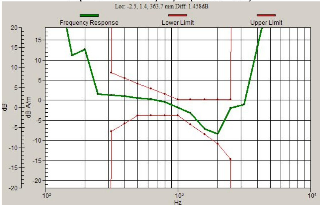
Graph 4: CDMA 1900 Frequency Response with Battery 2
