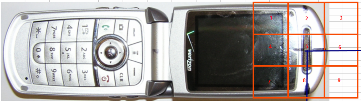
Figure A3-6. Phone Open – 5cm x 5cm grid for Near Field Measurements
