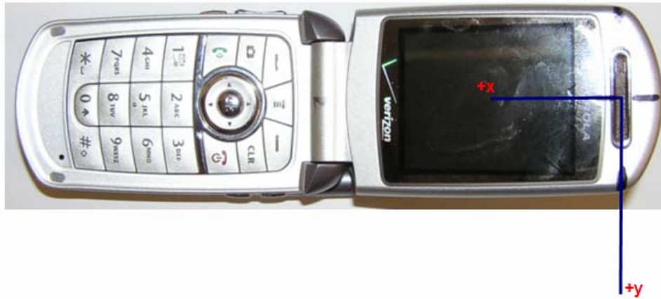
Figure A2-2. Phone Open – Coordinate Axis for T-coil Measured Point Location
