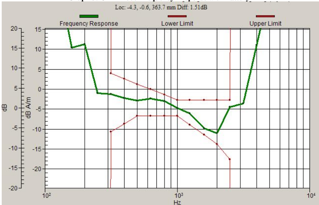
Graph 3: CDMA 800 Frequency Response with Battery 2
