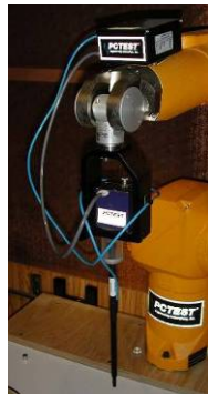
Figure 10 SPEAG Robotic System
