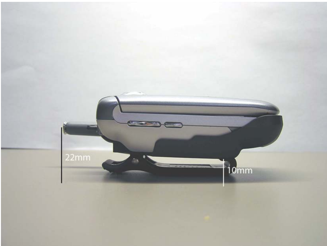
Figure 10. Side of Phone in Holster with Antenna Retracted and Extended Battery cover
