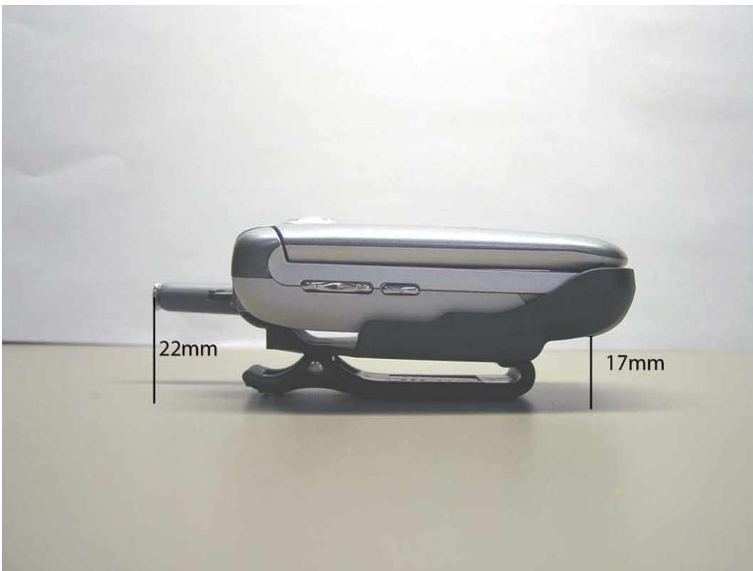
Figure 8. Side of Phone in Holster with Antenna Retracted and Standard Battery cover
