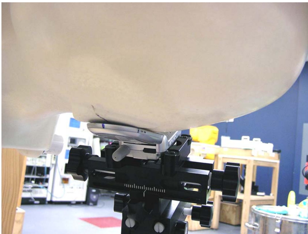
Figure 6. Phone Against the Head Phantom (Back View - Cheek Touch)
