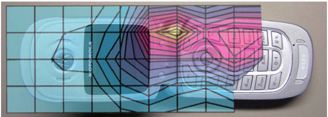
Figure 2. Typical 1900MHz Head Adjacent Contour Overlaid on Phone (Cheek Touch)
