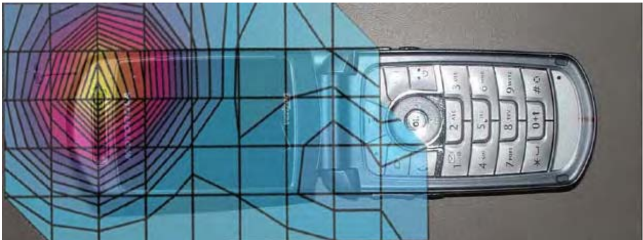
Figure 6. Typical 1900MHz Head Adjacent Contour Overlaid on Phone with Antenna Extended (15 ° Tilt)
