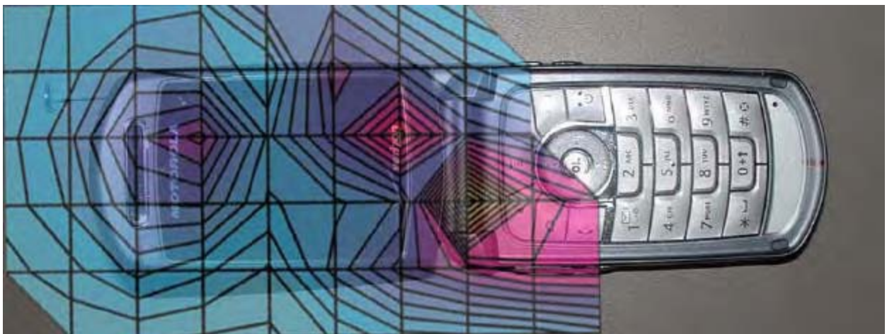
Figure 2. Typical 1900MHz Head Adjacent Contour Overlaid on Phone with Antenna Extended (Cheek Touch)
