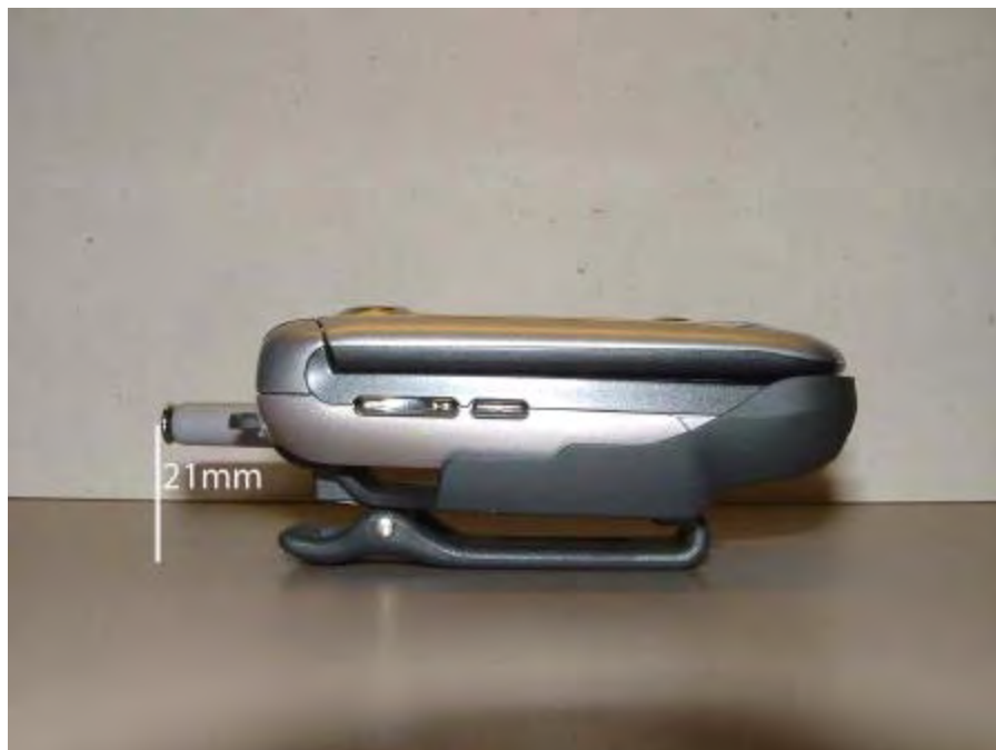
Figure 21. Side View; Phone in SYN0912A with Antenna Retracted
