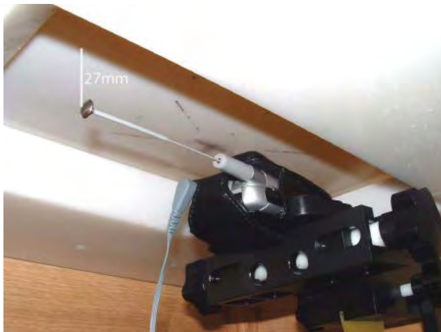
Figure 36. Phone in CHYN4459A Against the Flat Phantom with Antenna Extended
