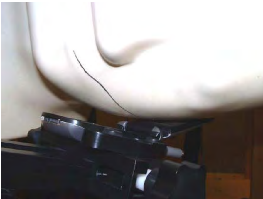
Figure 27. Phone Against the Head with Antenna Retracted (Front View – Cheek Touch)
