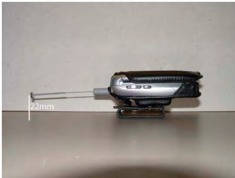
Figure 23. Side View; Phone in SYN9766A and SYN8631A with Antenna Extended
