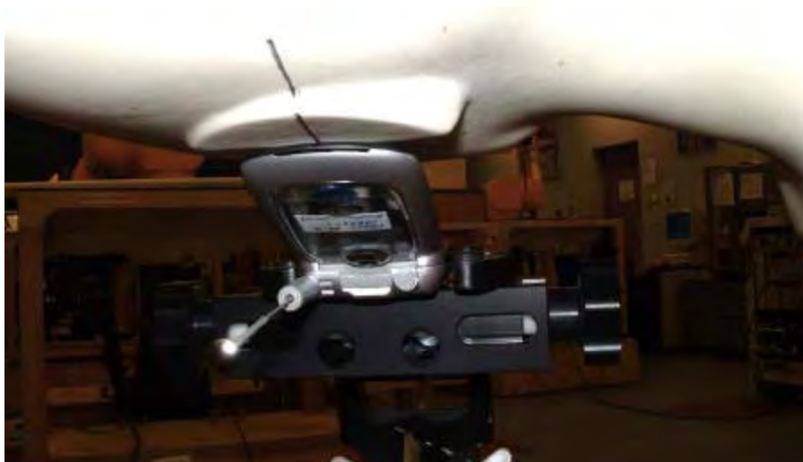
Figure 34. Phone Against the Head with Antenna Extended (Back View – 15°Tilt)
