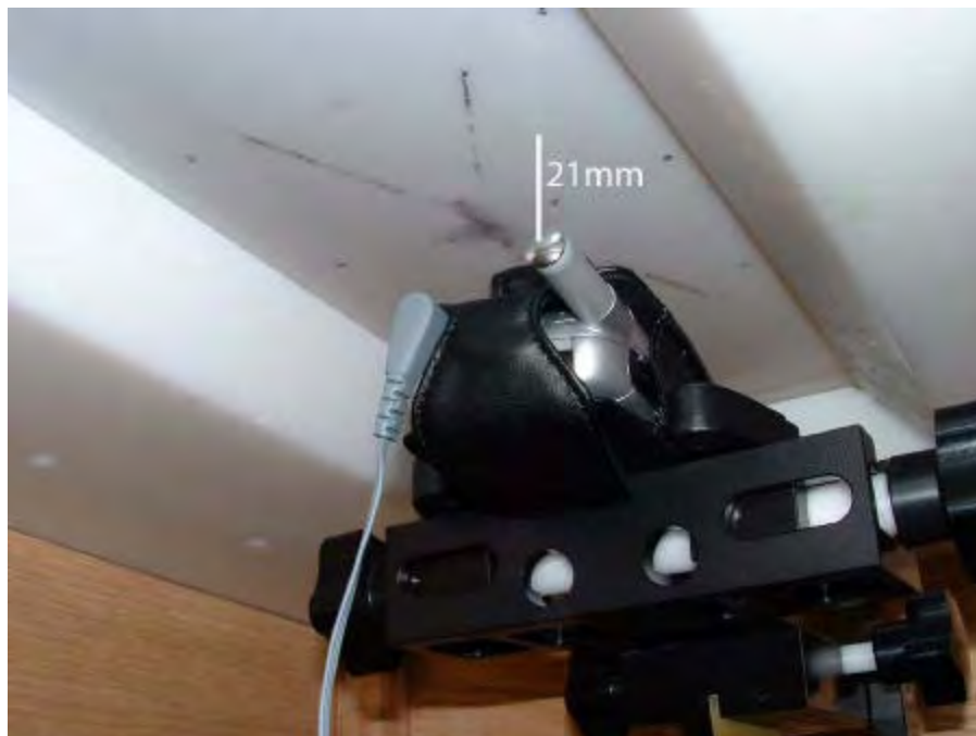
Figure 35. Phone in CHYN4459A Against the Flat Phantom with Antenna Retracted
