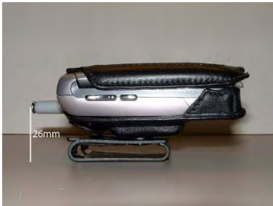
Figure 23. Side View; Phone in SYN9766A and SYN8631A with Antenna Retracted
