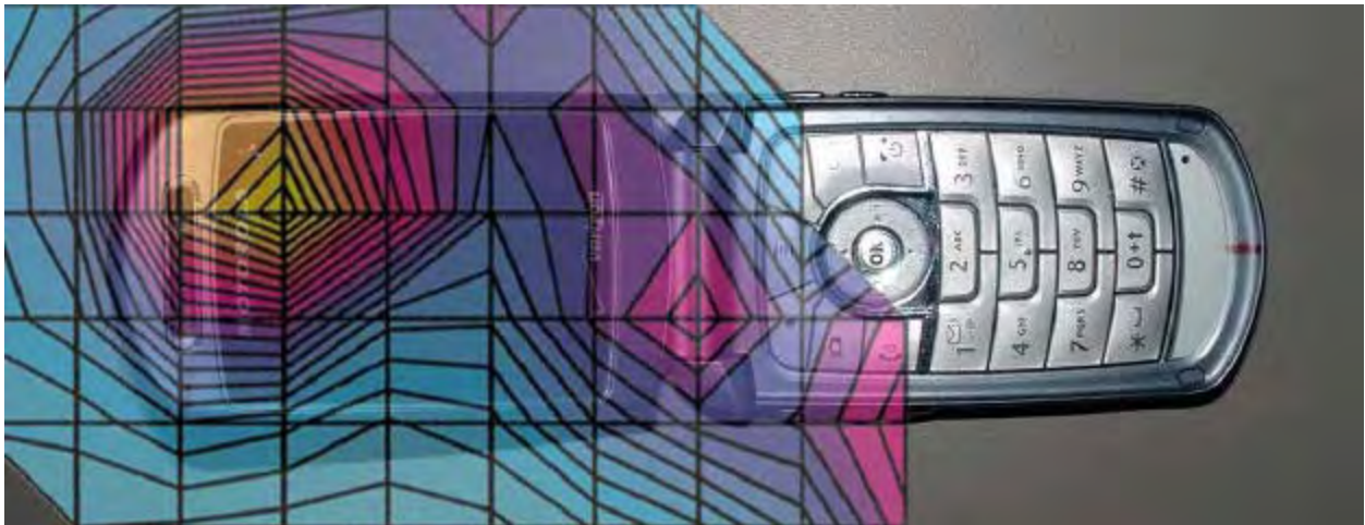
Figure 8. Typical 1900MHz Head Adjacent Contour Overlaid on Phone with Antenna Retracted (15 ° Tilt)
