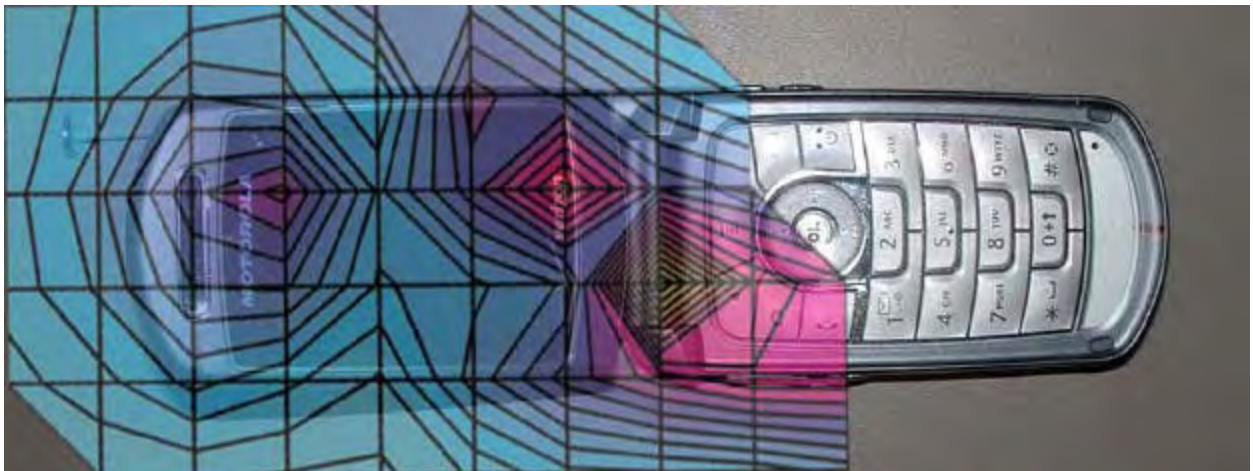
Figure 2. Typical 1900MHz Head Adjacent Contour Overlaid on Phone with Antenna Extended (Cheek Touch)
