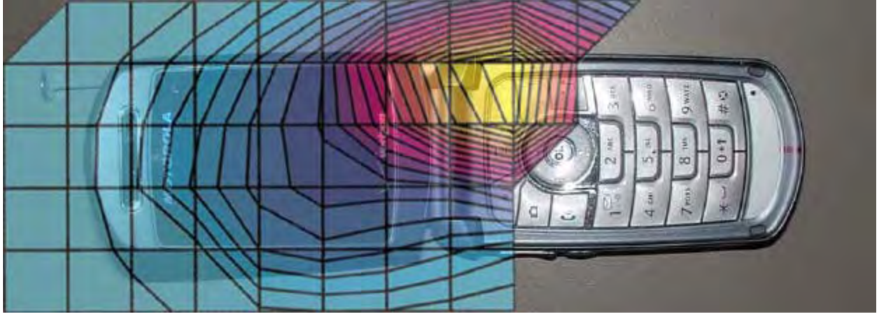
Figure 1. Typical 800MHz Head Adjacent Contour Overlaid on Phone with Antenna Extended (Cheek Touch)
