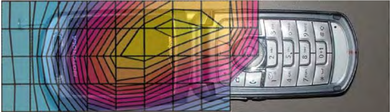
Figure 5. Typical 800MHz Head Adjacent Contour Overlaid on Phone with Antenna Extended (15 ° Tilt)
