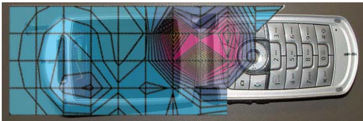
Figure 2. Typical 1900MHz Head Adjacent Contour Overlaid on Phone with Antenna Extended (Cheek Touch)
