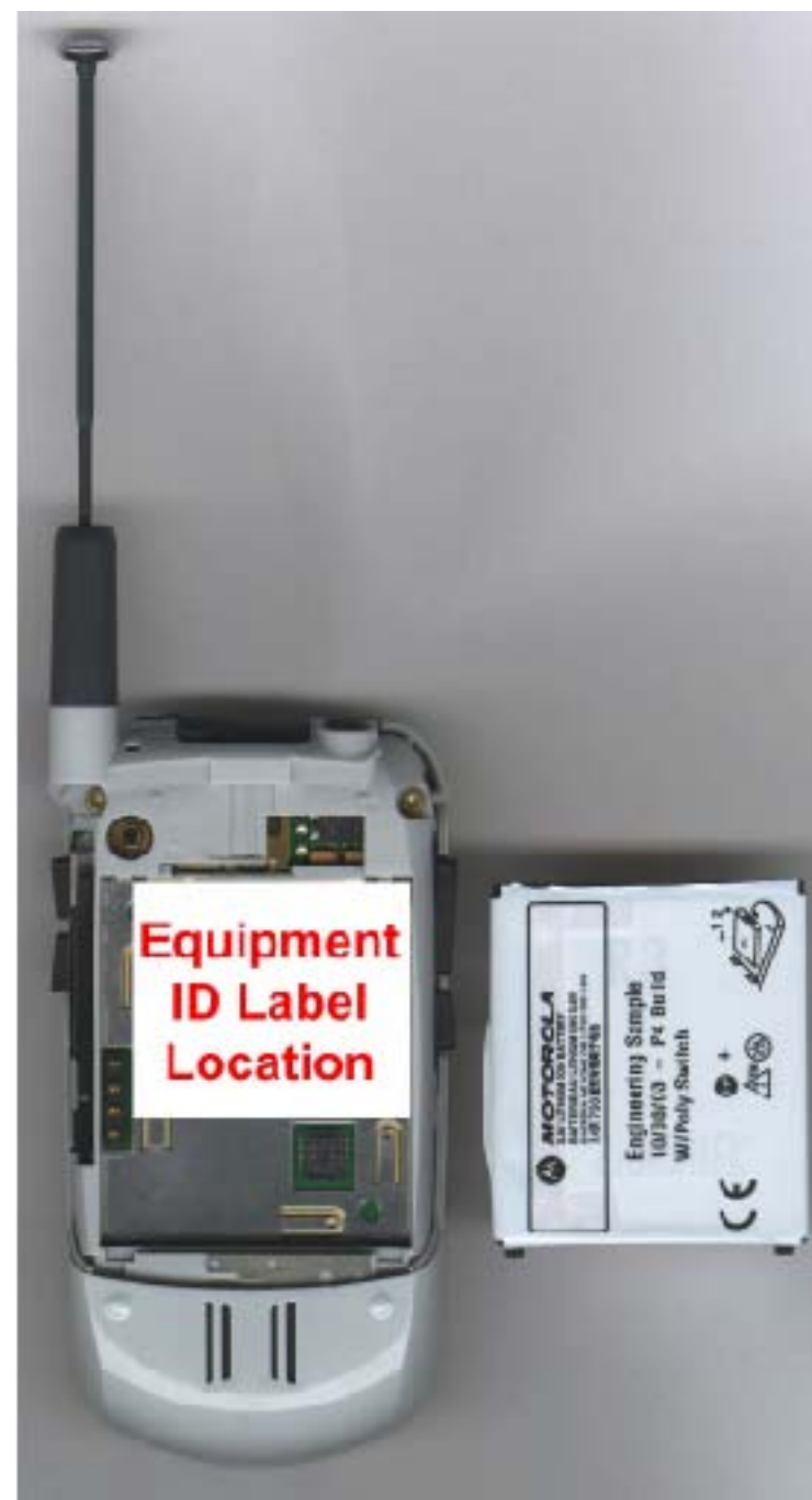
Rear View with Battery Removed Showing ID Label
