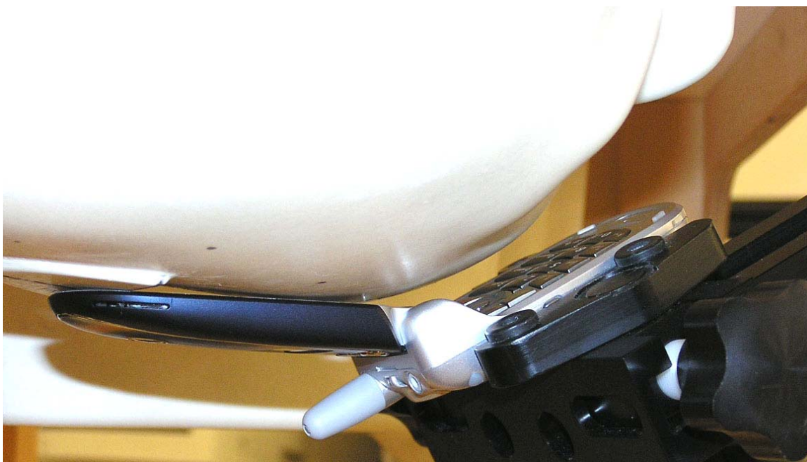
Figure 4. Phone Against the Head Phantom (Cheek Touch)
