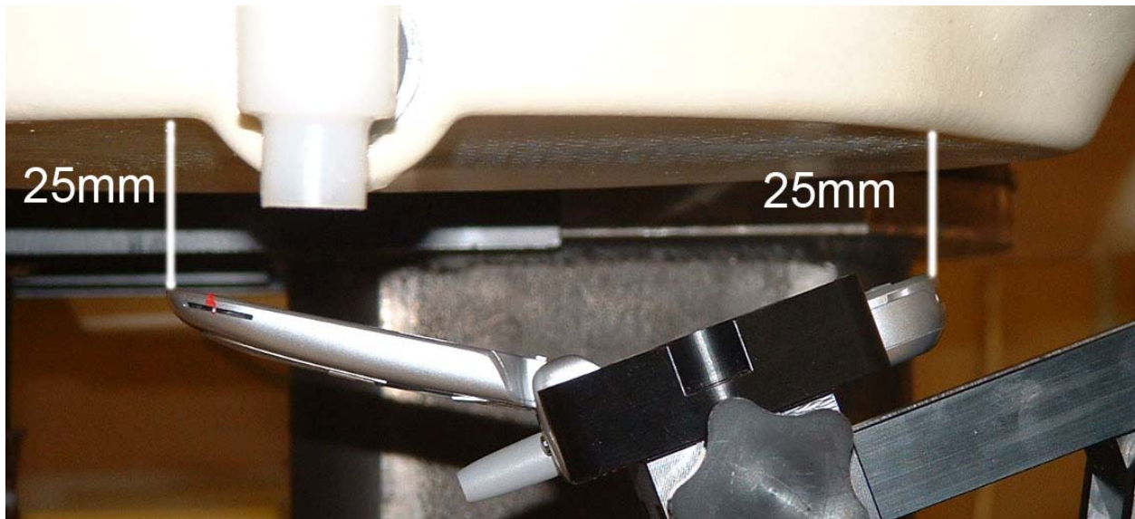
Figure 6. Phone Against the Flat Phantom (PTT position)
