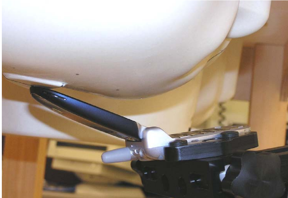
Figure 5. Phone Against the Head Phantom (15°Tilt)
