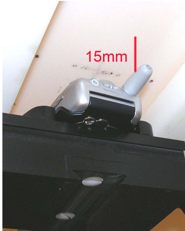
Figure 7. Phone Against the Flat Phantom (Body)
