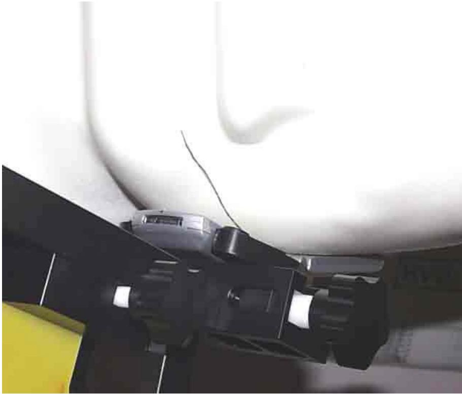
Figure 10. Phone Against the Head Phantom (Front View - Cheek Touch)
