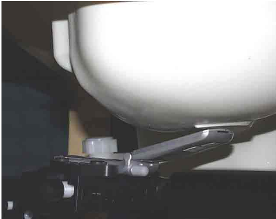
Figure 13. Phone Against the Head Phantom (Back View – 15°Tilt)
