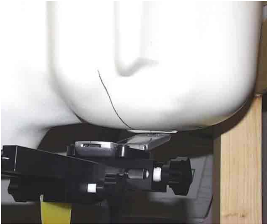
Figure 12. Phone Against the Head Phantom (Front View – 15°Tilt)
