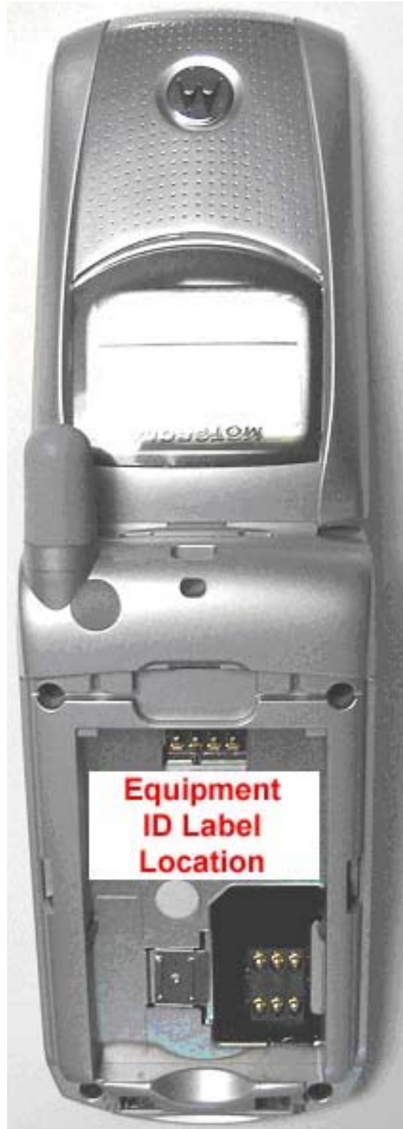
BACK VIEW with Battery removed to show Equipment ID Label
