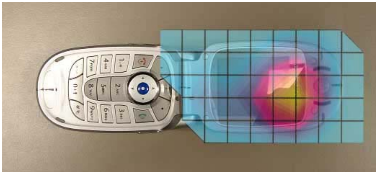
Figure 4. Typical 1900MHz Right Head Adjacent Contour Overlaid on Phone with Antenna Fixed (15° Tilt)
