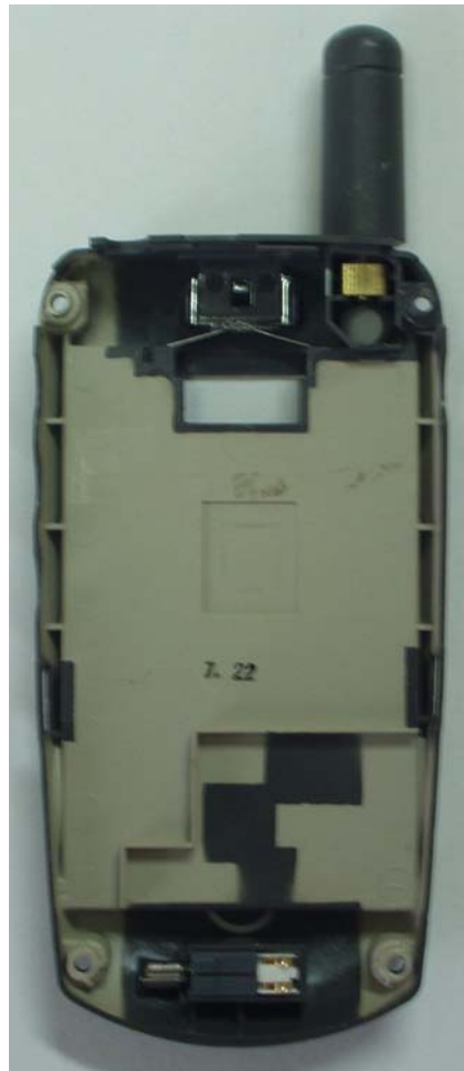
Rear Housing Internal View
