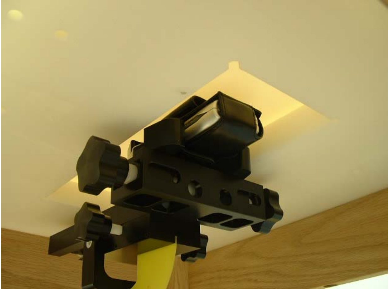
Phone in leather case against the flat phantom
