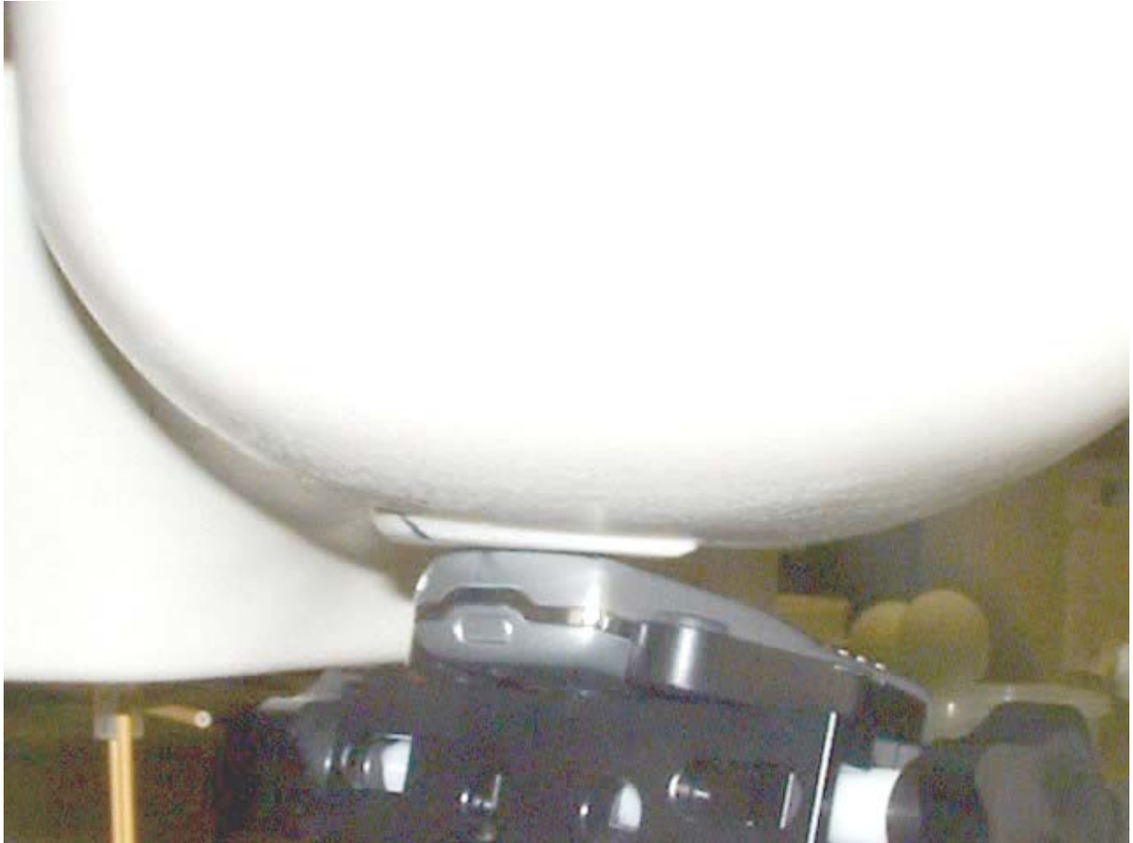
Phone Placed Against Phantom Head in 15 Degree Tilt Position
