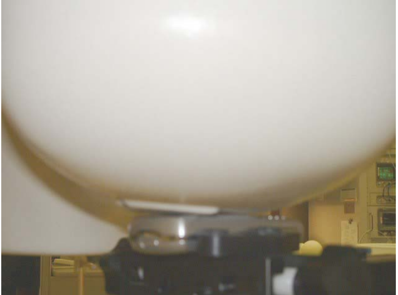
Phone Placed Against Phantom Head in Check Touch Position
