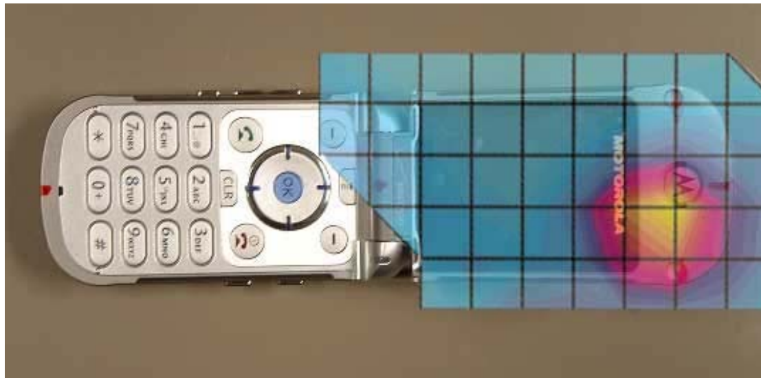
Figure 4. Typical 1900MHz Left Head Adjacent Contour Overlaid on Phone with Antenna Retracted (15°Tilt)
