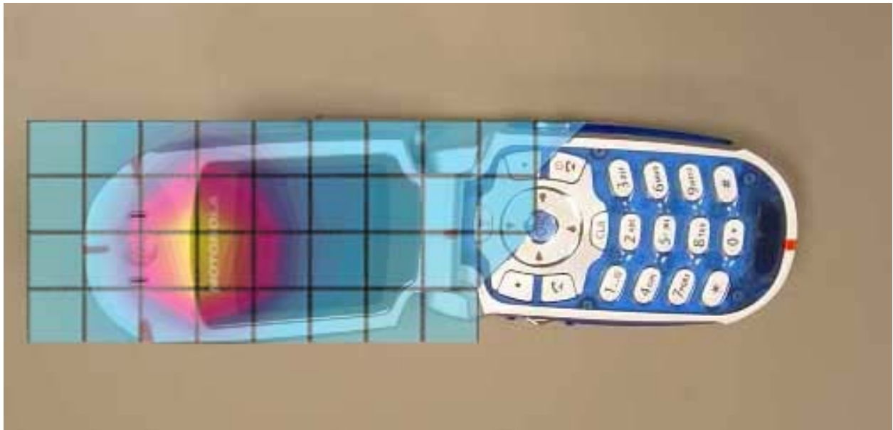
Figure 4. Typical 1900MHz Right Head Adjacent Contour Overlaid on Phone with Antenna Fixed (15° Tilt)
