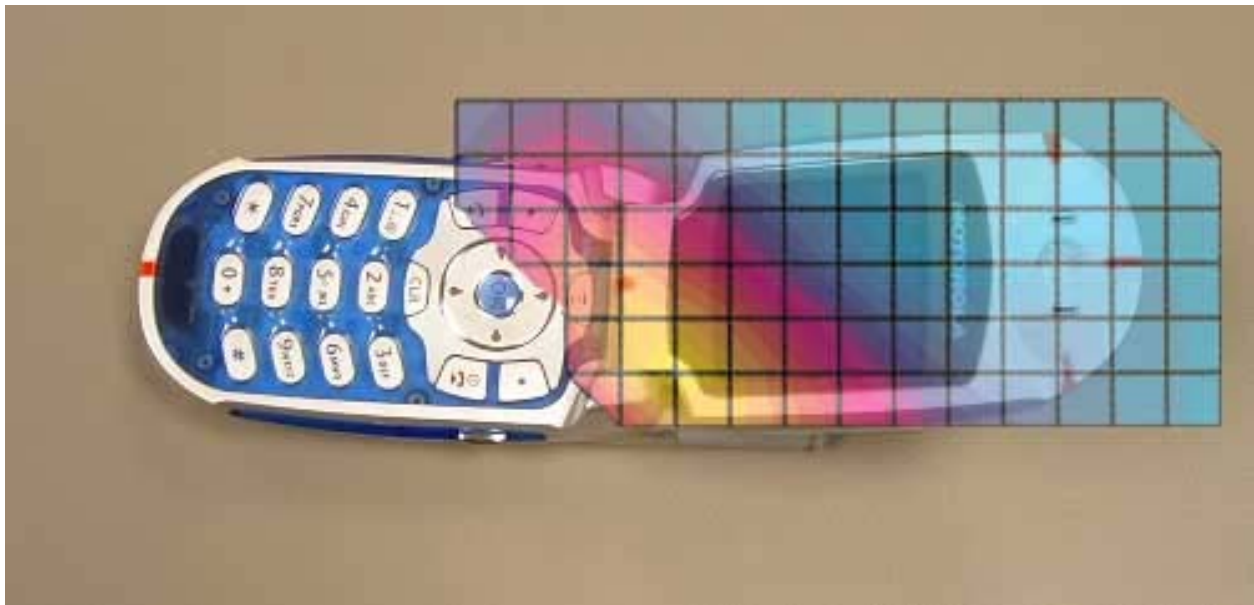
Figure 2. Typical 800MHz Left Head Adjacent Contour Overlaid on Phone with Antenna Extended (15° Tilt Position)
