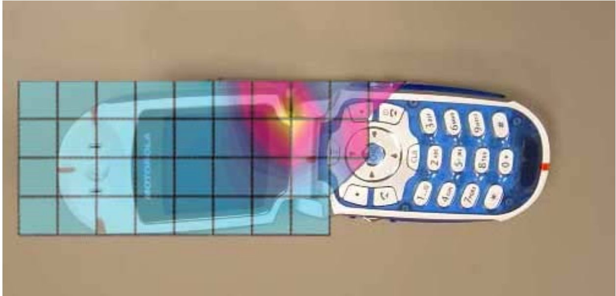
Figure 3. Typical 1900MHz Right Head Adjacent Contour Overlaid on Phone with Antenna Fixed (Cheek Touch)
