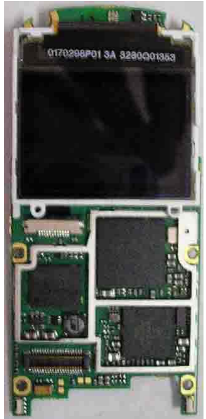
Front View Shields Removed
