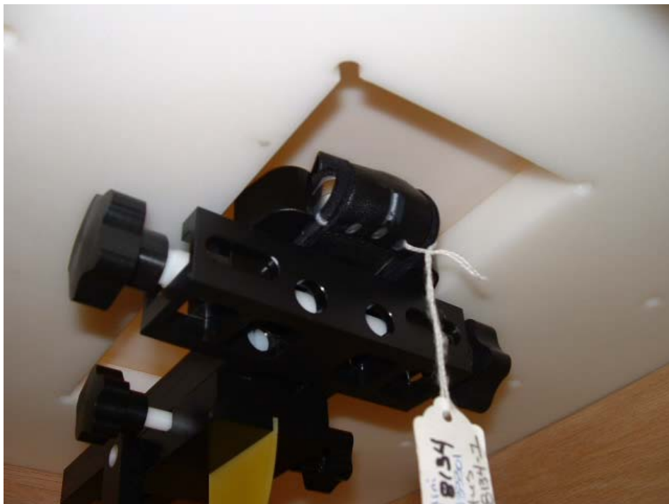
Figure 4. MN33301 Case with SYN8631A Belt Clip in Test Position
