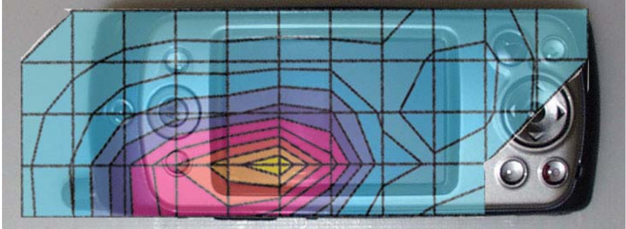
Figure 1. Typical 1900MHz Head Adjacent Contour Overlaid on Phone (Cheek Touch)
