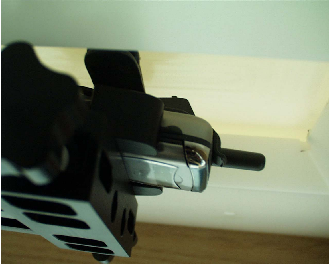
Figure 4. DUT below “Twin Tub” Body-Worn Measurement Phantom
