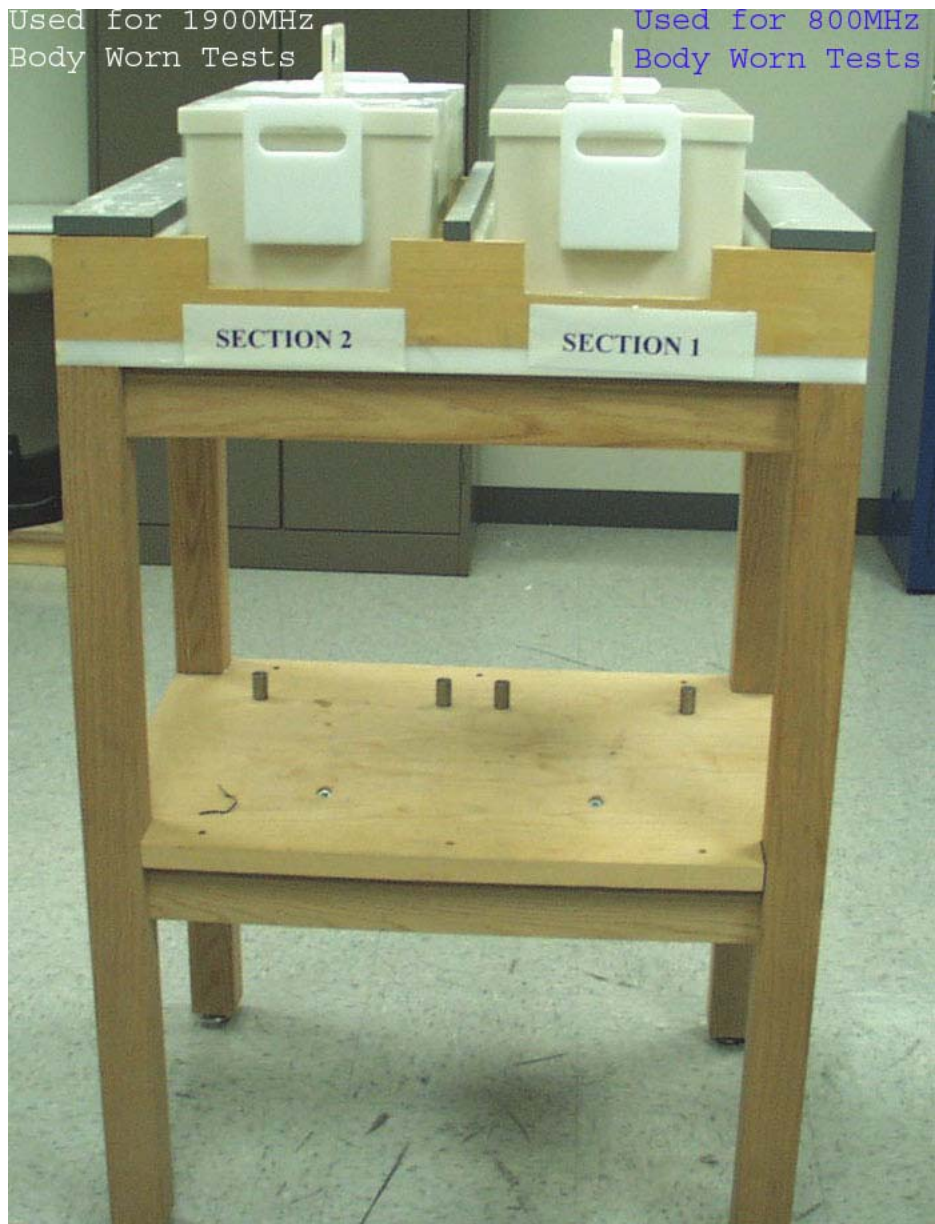
Figure 1. "Twin Tub" Body-Worn Measurement Phantoms and Fixture.
