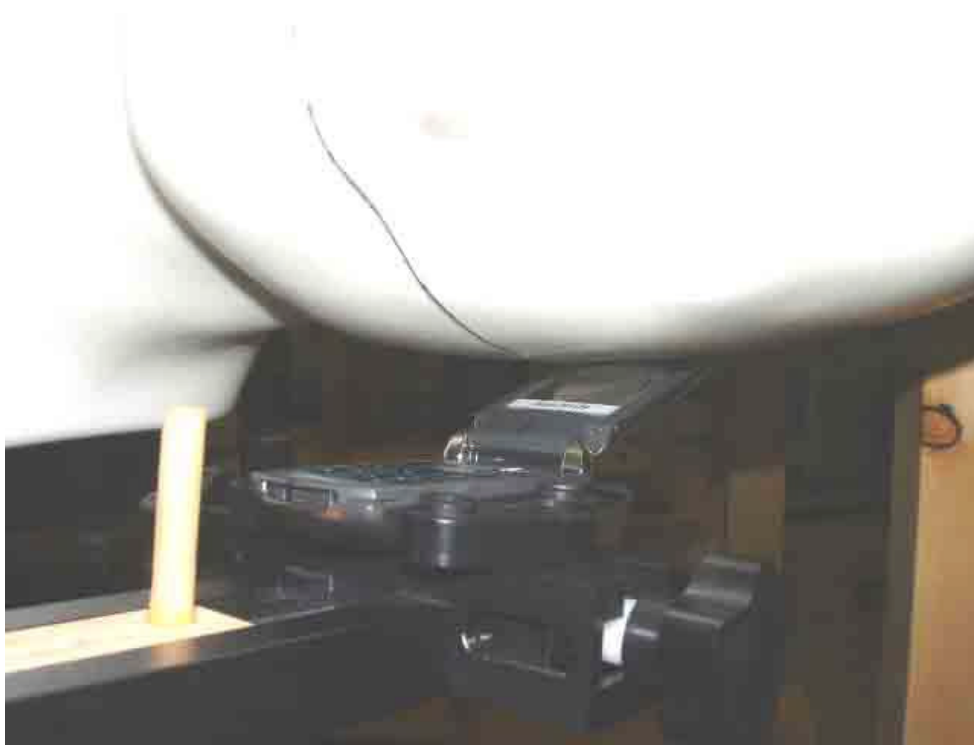
Figure 13. Phone Against the Head (15° Tilt) Front View
