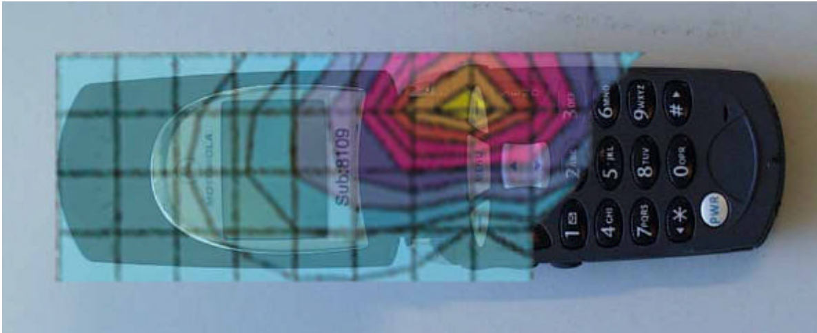
Figure 1. Typical 800 MHz Right Head Adjacent Contour Overlaid on Phone with Antenna Fixed (Cheek Touch)
