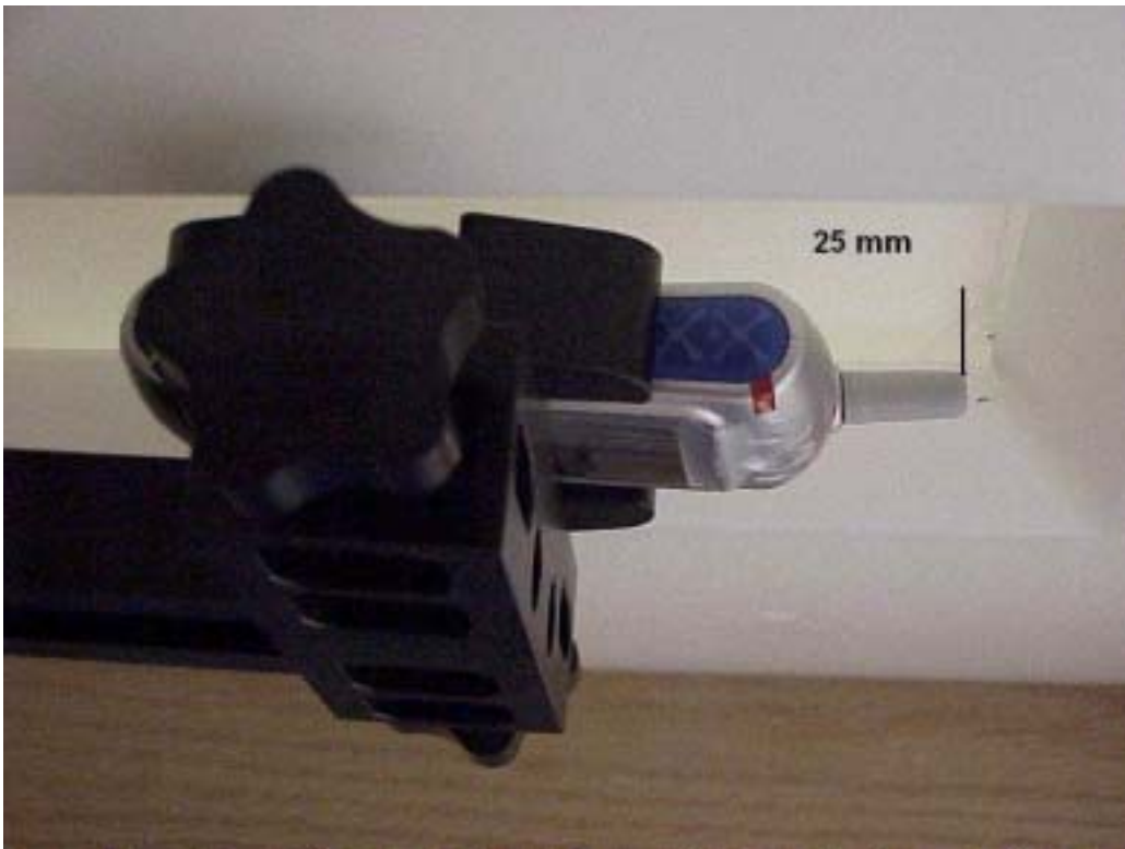
Figure 10. Phone in the positioner distanced 1 inch away from the flat phantom (Antenna Fixed)
