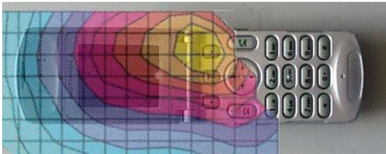
Figure 6. Typical 800MHz Head Adjacent Contour Overlaid on Phone with Antenna Retracted (15 ° Tilt)
