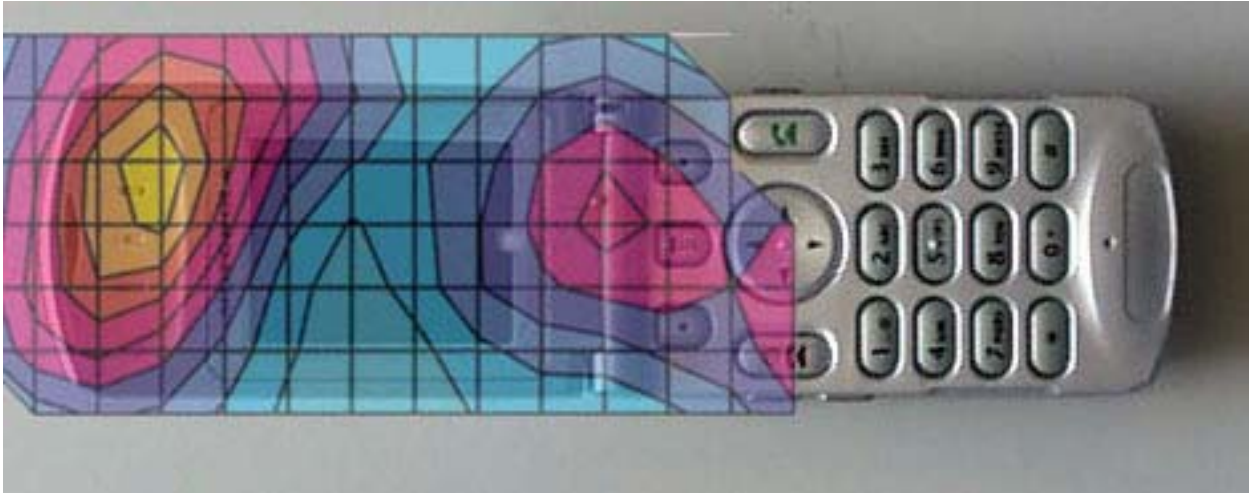
Figure 7. Typical 1900MHz Head Adjacent Contour Overlaid on Phone with Antenna Extended (15 ° Tilt)
