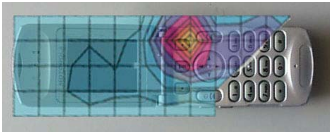
Figure 2. Typical 1900MHz Head Adjacent Contour Overlaid on Phone (Cheek Touch)
