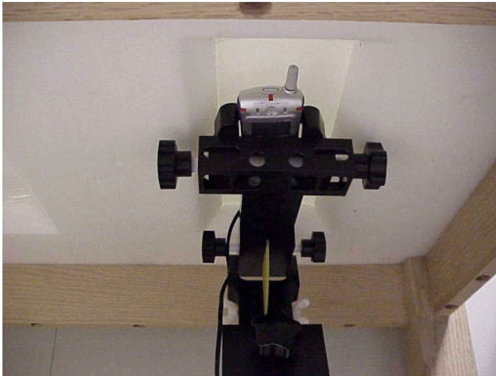
Figure 11. Phone in the positioner distanced 1 inch away from the flat phantom with Head Set Attached (Antenna Fixed)
