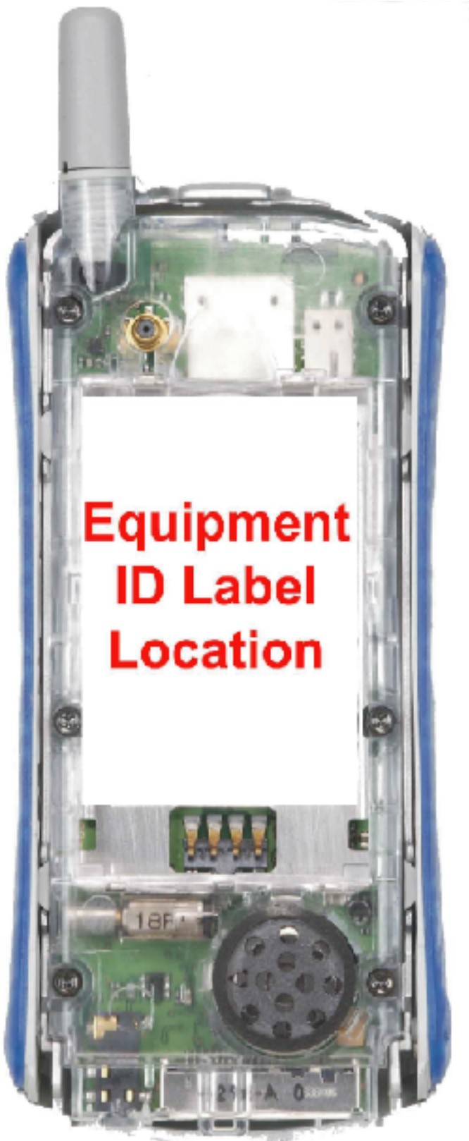
Rear View, with Battery Removed to Show Equipment ID Label
