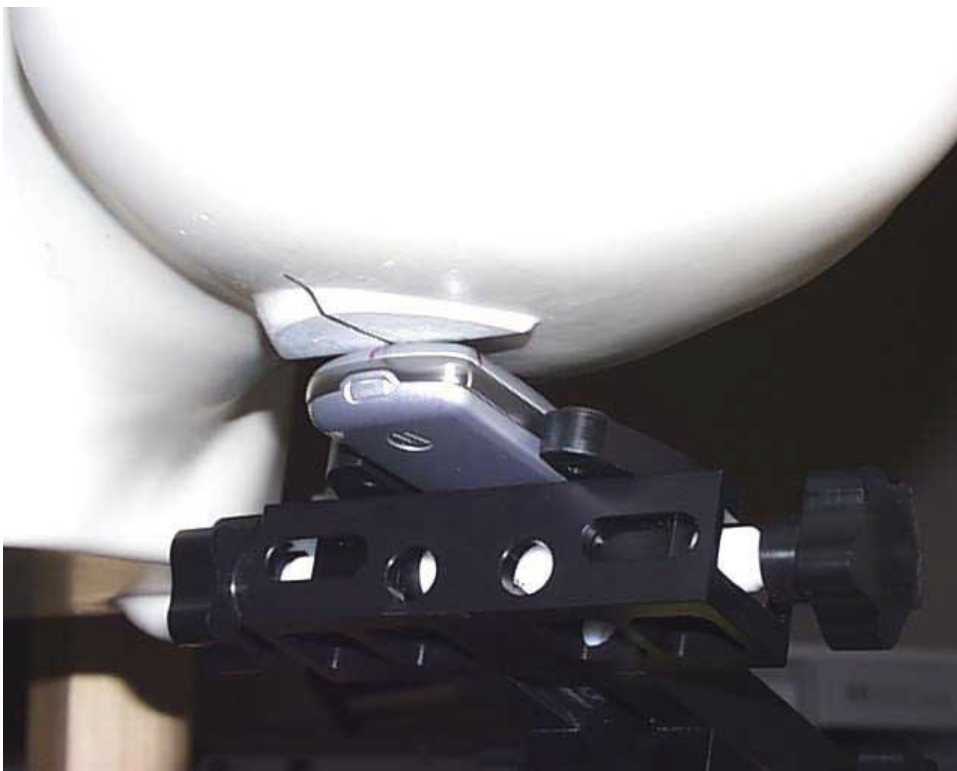
Figure 15. Phone Against head phantom (15°Tilt) (Back View)
