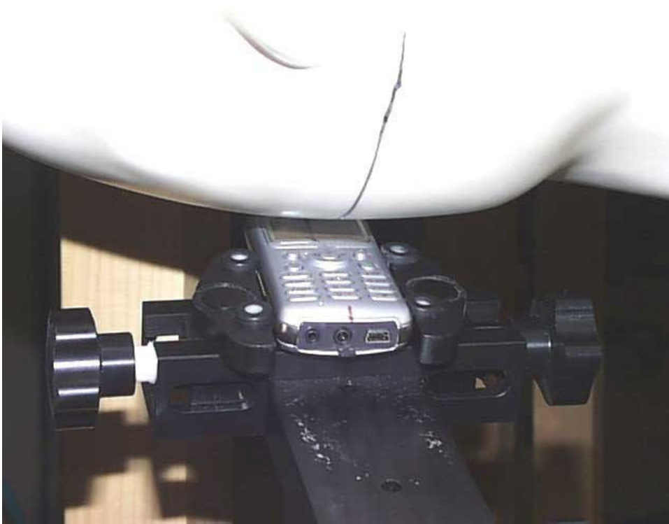
Figure 14. Phone Against head phantom (15°Tilt) (Front View)
