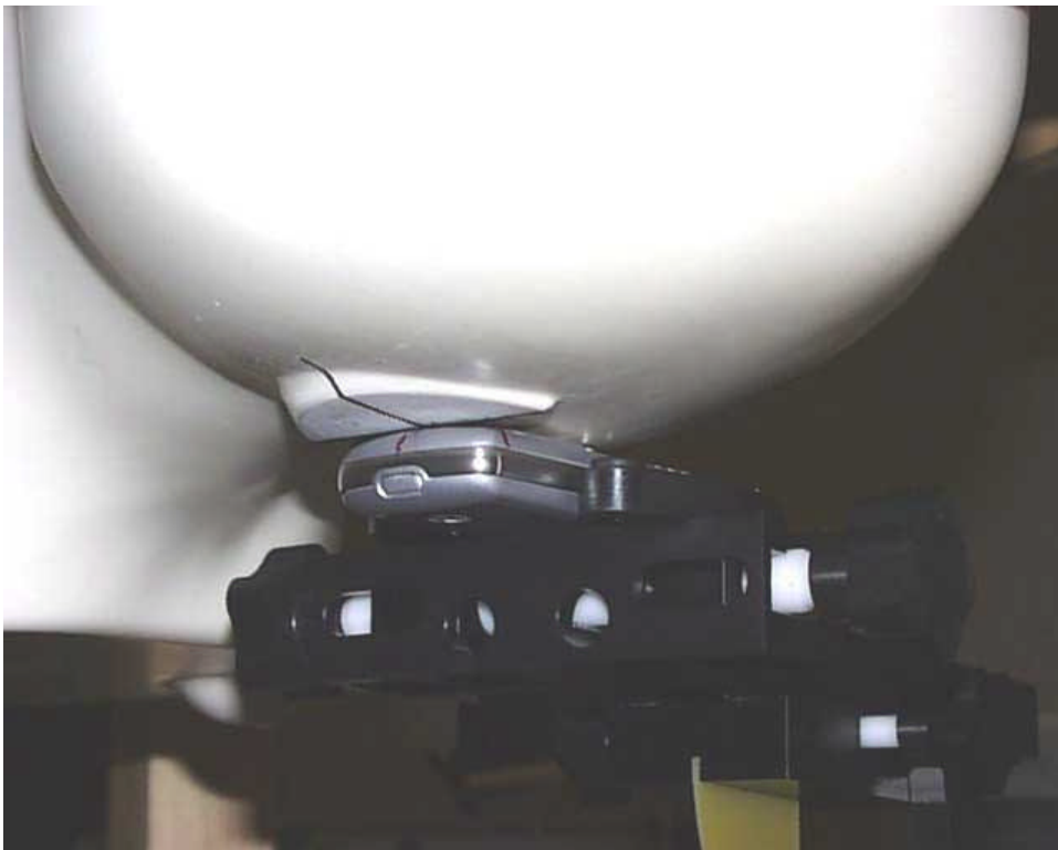
Figure 13. Phone Adjacent to head phantom (Back View)
