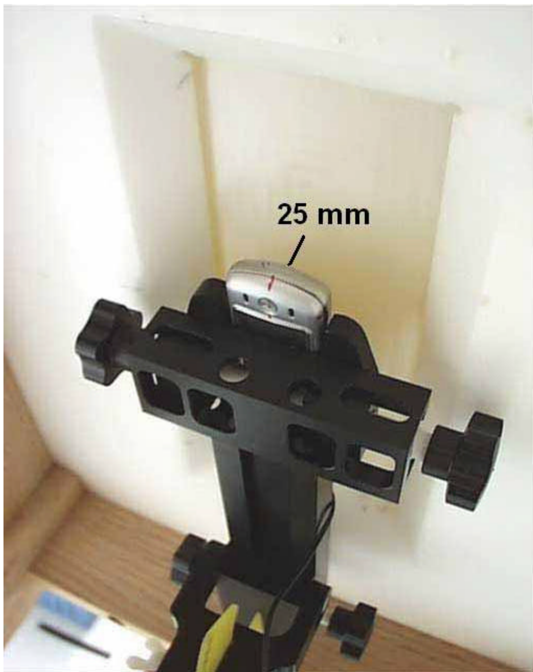
Figure 11. Separation Distance between Phone and Flat Phantom
