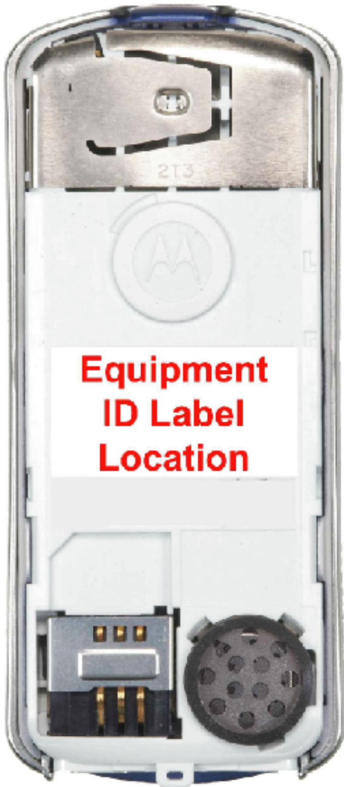
Rear View with housing removed to show equipment ID label
